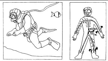
Figure 8. Schematic illustration of a hot water suit. From: Ornhagen, 1998.
