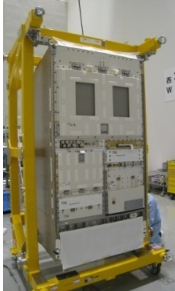
Multi-purpose Small Payload Rack (MSPR)
