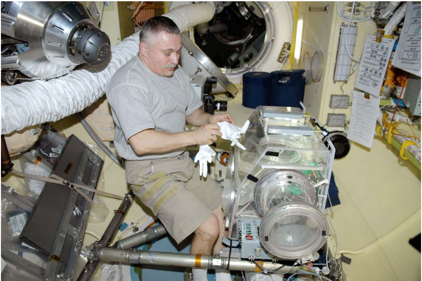
Russian cosmonaut Fyodor Yurchikhin, Expedition 25 flight engineer, prepares the Russian Glavboks-S (Glovebox) for the bioscience experiment ASEPTIC (BTKh-39) in the Poisk Mini-Research Module 2 (MRM2) of the International Space Station.
