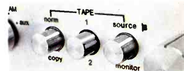
Two completely independent tape monitors.
