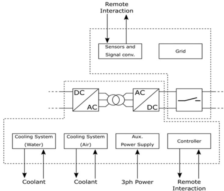
Figure 12: Boundary definition for MV7000 DAB Converter.
