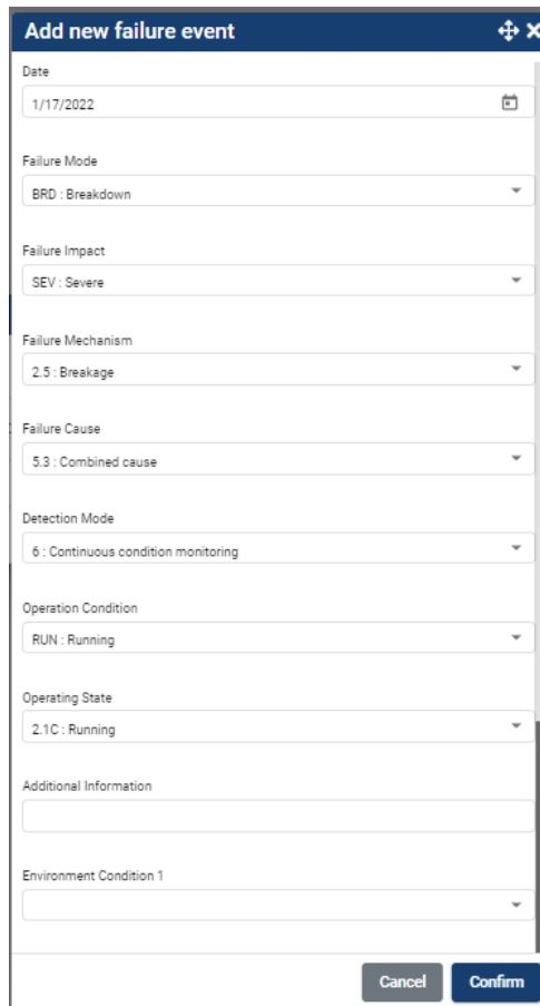
Figure 18: Add a new Failure Event.
