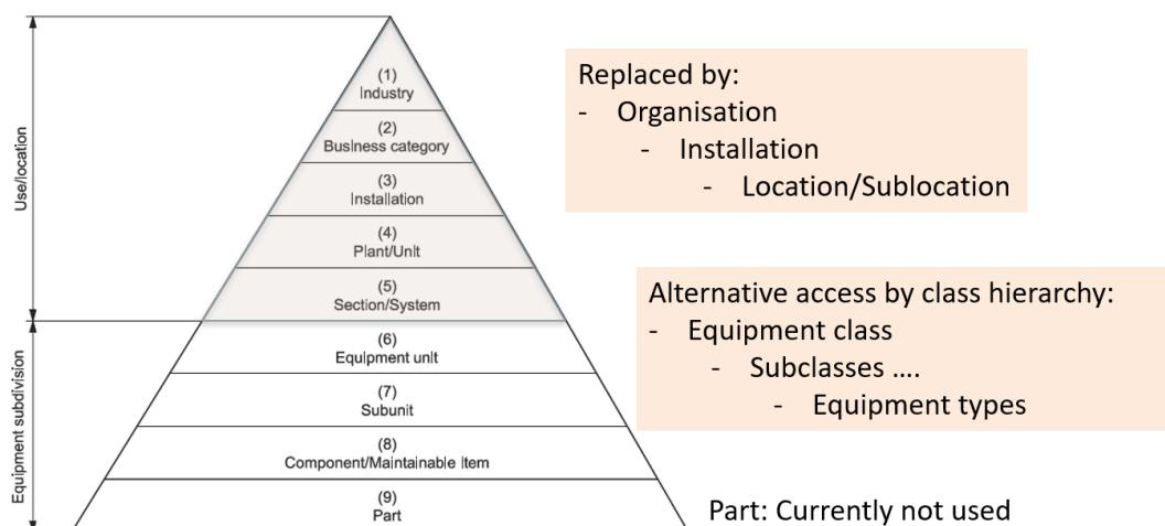
Figure 8: Model for describing the structure of a catalogue.
