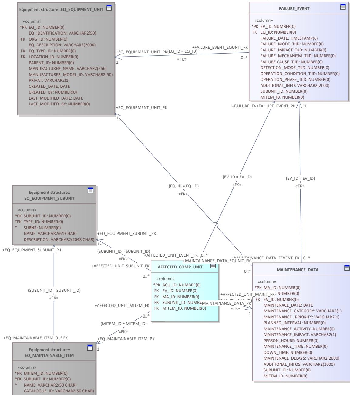
Figure 31: Model Failure and Maintenance.
