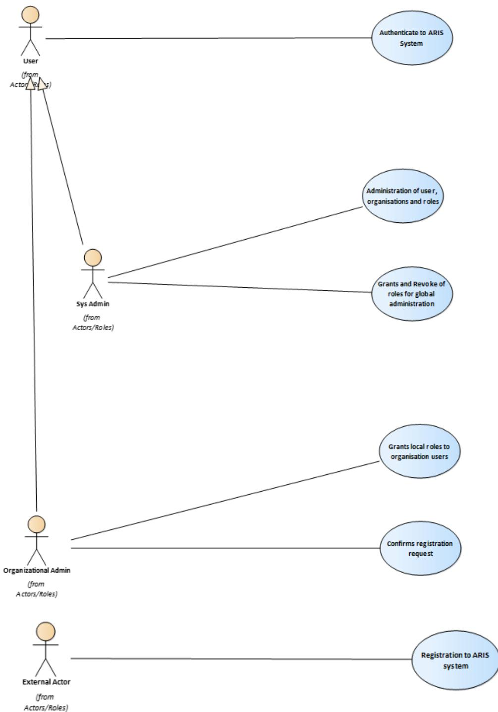
Figure 26: Use Case diagram for the administration of actors within the system.
