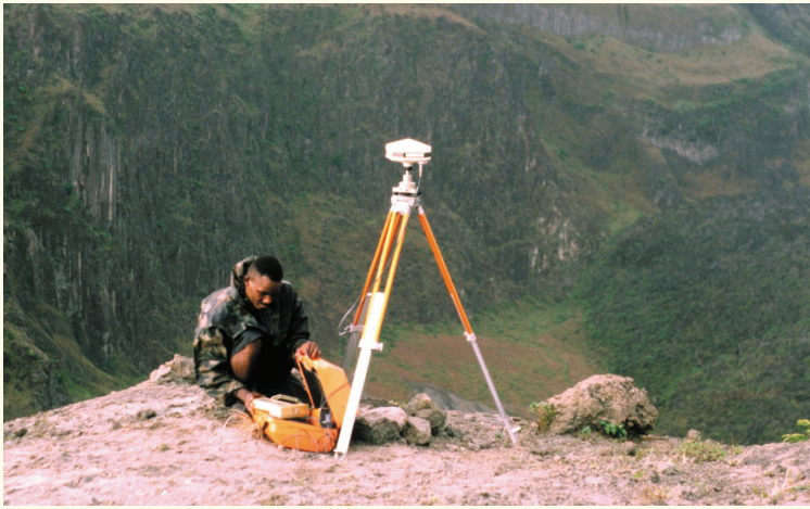
Technician from the Soufrière Monitoring Unit assisting with GPS measurements at the summit of the Soufrière Volcano
