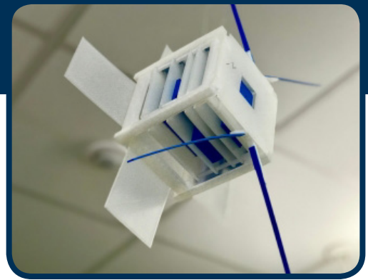
The approximately four-inch CubeSat that was built by Old Dominion students will be launched from the International Space Station later this year.
