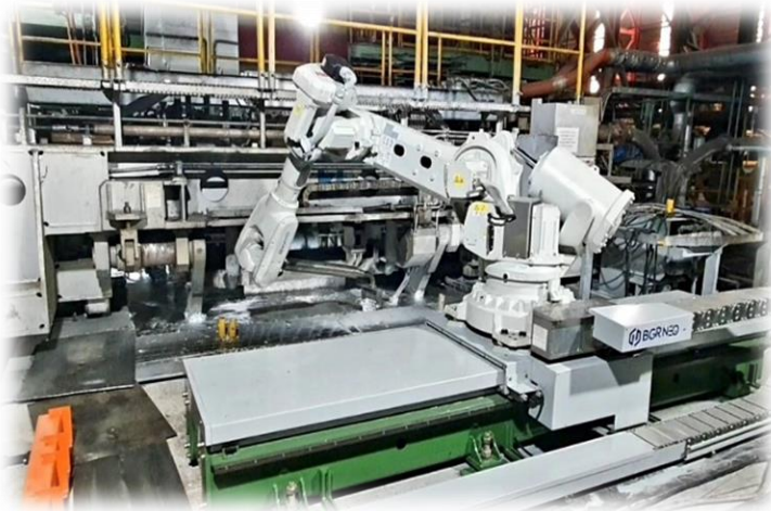
CRM-2: Dross cleaning robot for human safety
