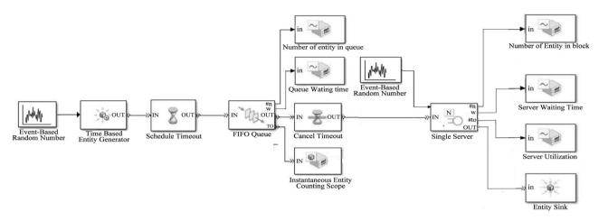
Figure 8. Simulink model.
