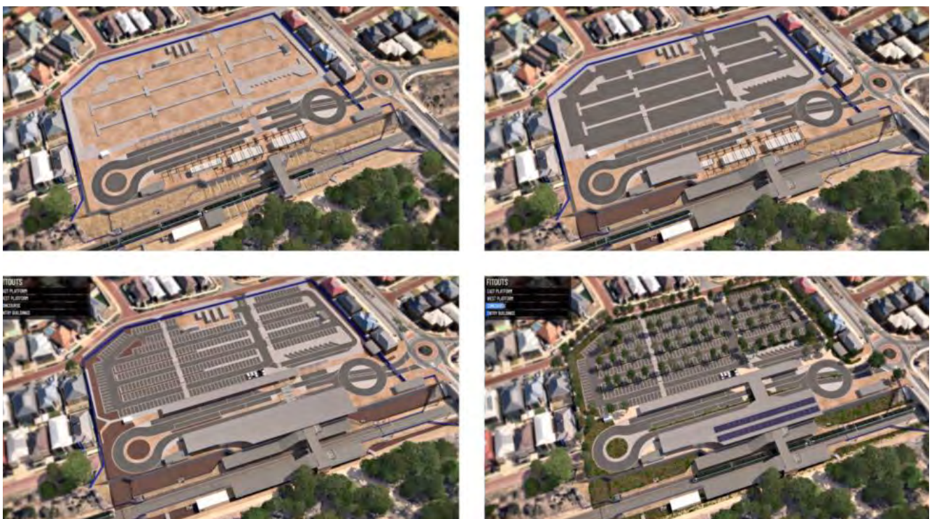
Figure 17: Staging Plans (ADCO Constructions 2021)
