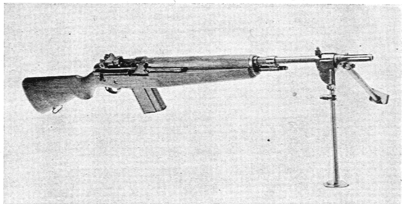
Heavy-barrel form is the Automatic Rifle M15. Its special features are a heavy barrel, muzzle bipod, butt hook, and heavier stock. The M15 will always be fitted with the change lever permitting full-automatic fire. Its weight is 14.1 lbs., or 6.7 lbs. less than the Browning automatic rifle (BAR) which it replaces
