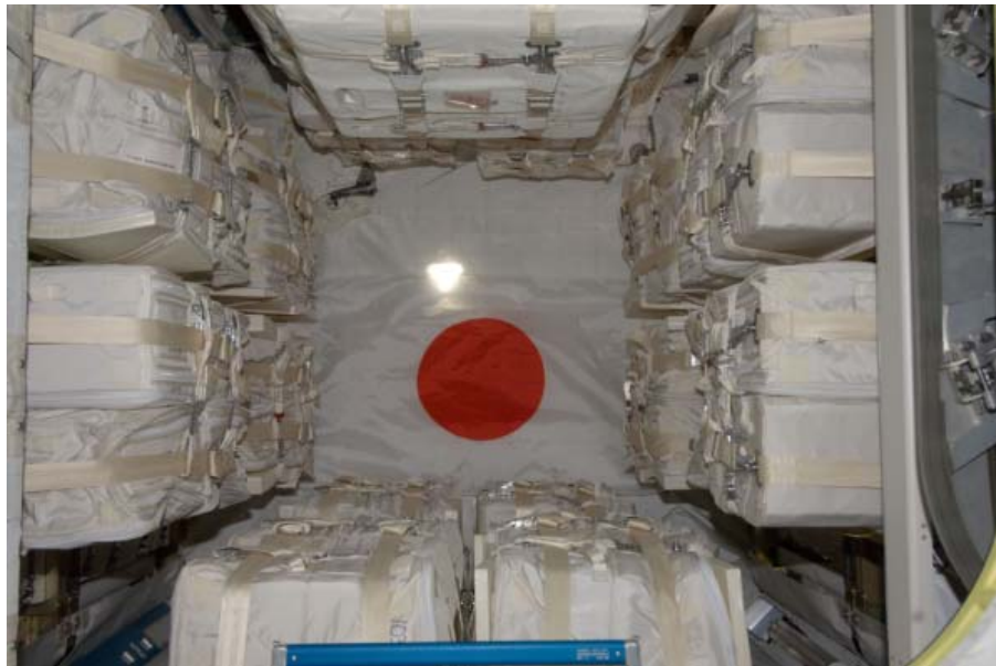
Inside of the HTV PLC (HTV1)
