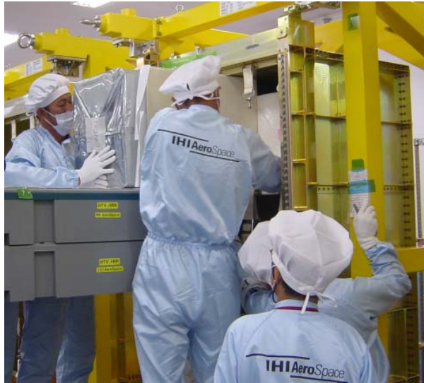
Fig. 1.7.1-4 CTBs Being Installed in a HRR
