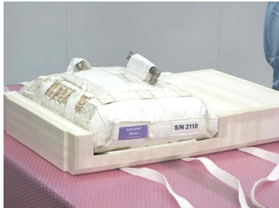
Contingency Water Container-Iodine (CWC-I) mounted on a cushion plate
