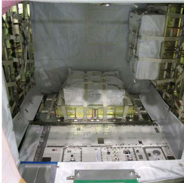
The above picture was taken during cargo loading activities (HTV2) Fig. 1.7-1 HTV Pressurized Logistics Carrier (PLC)
