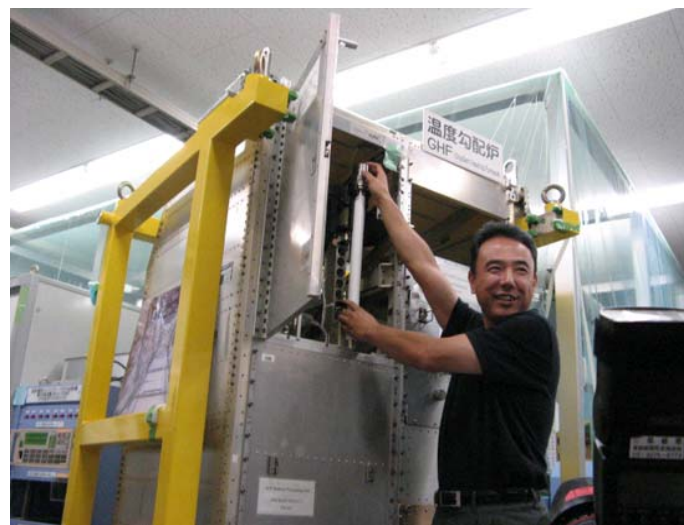
Fig. 1.7.1-8 Astronaut Furukawa and the Gradient Heating Furnace (GHF) Astronaut Furukawa pulling out a sample cartridge from the GHF during a preflight training session
