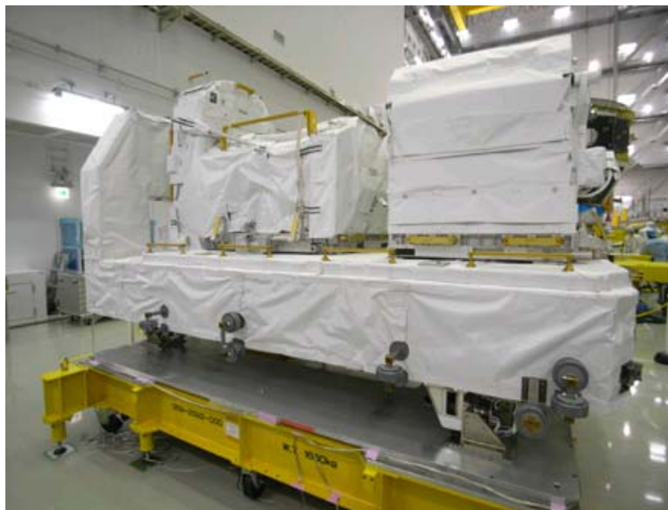
Two unpressurized payloads (or ORUs) are installed on the EP Fig. 1.7-2 HTV Exposed Pallet (EP) (HTV2)
