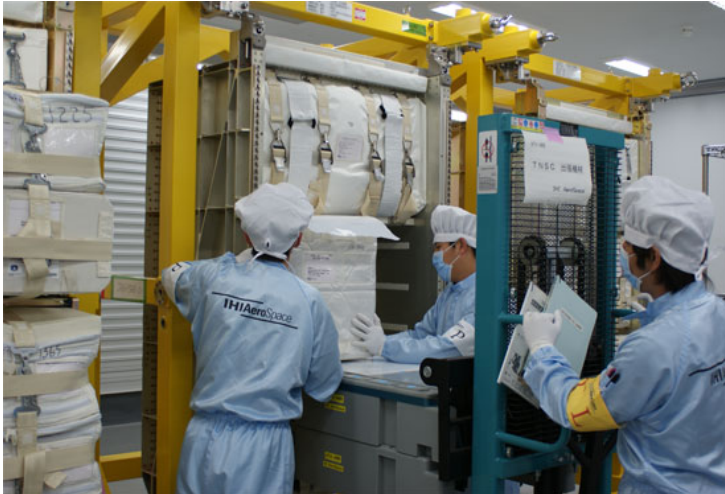
Cargo Transfer Bags (CTBs) Being Installed in the HTV Resupply Rack (HRR)
