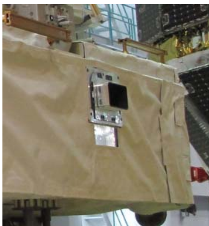
Fig. 2.4.3-6 HTV Berthing Camera System (HBCS)
