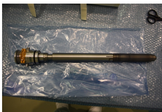
Fig. 1.7.1-11 Test Sample Cartridge for In-Flight GHF Checkout
