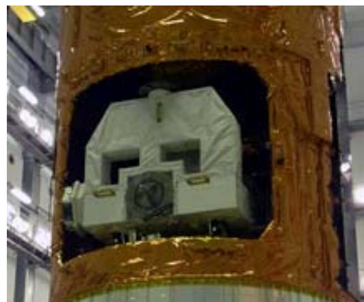
Fig. 2.4.2-3 EP Installed into the ULC (HTV2)
