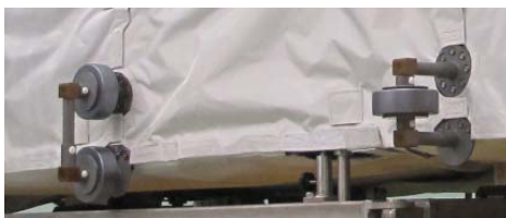
Fig. 2.4.2-4 Enlarged View: Opening of the ULC (HTV1) Wheel on the EP (HTV2)
