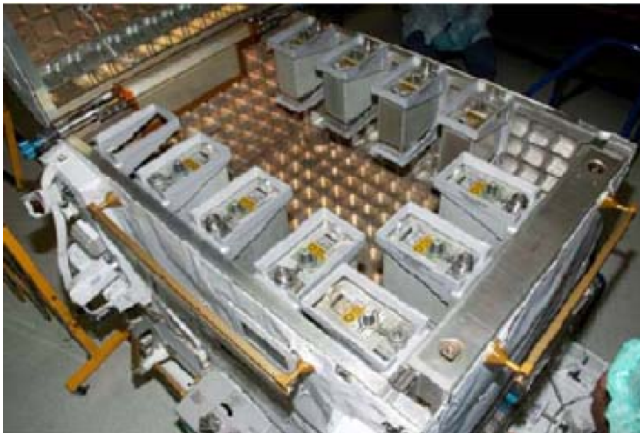
Fig. 1.7.2-4 Layout inside the CTC (STS-129) Boxes attached inside are spare RPCMs (Total of 10 units).
