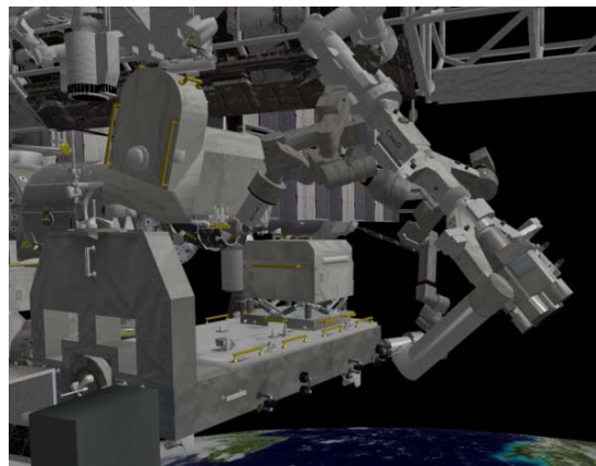
DEXTER (SPDM) Grappling the FHRC (Image)
