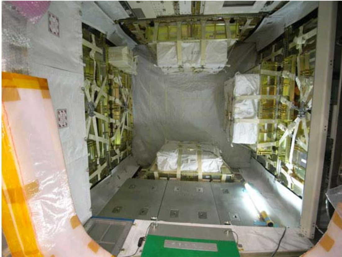
Fig. 2.4.1-3 Rack Layout inside the PLC (The above picture was taken during the cargo loading activities in preparation for the HTV2 Mission)
