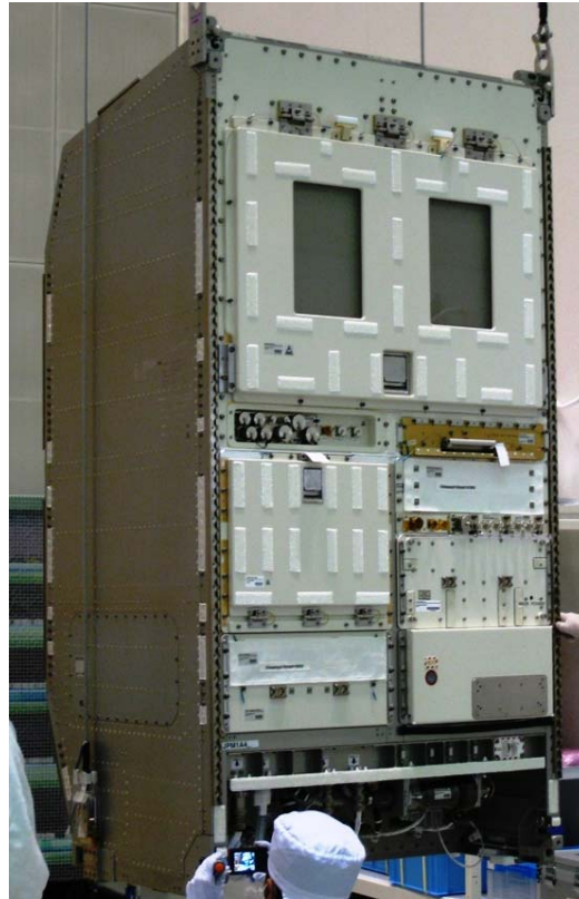
Fig. 1.7.1-12 Multi-purpose Small Payload Rack (MSPR)
