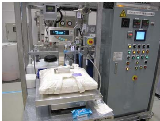
Fig. 1.3-3 Water Loading System Introduced at Tanegashima Space Center
