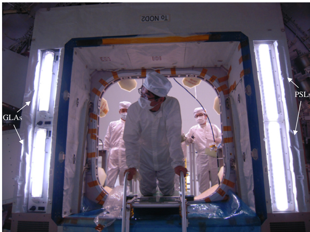
Fig. 1.3-1 New Locations of Lights on board the PLC (HTV2)
