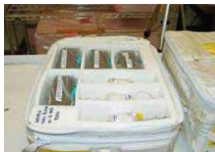
Food, daily commodities, and experiment samples are packed in the CTBs. The CTBs are installed in the HRRs
