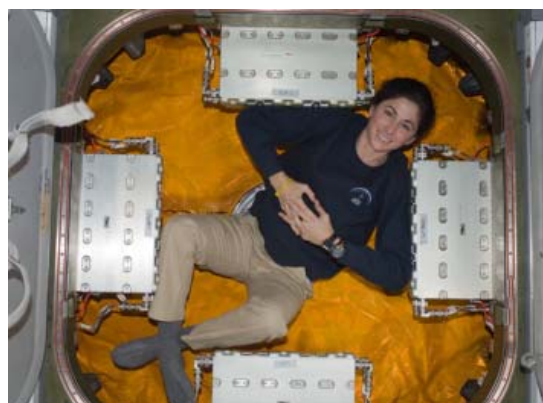
Four silver boxes seen in the picture are the CPAs
