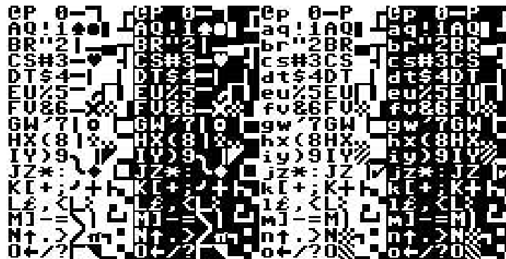
Figure 9. The Commodore 64 and 128 “PETSCII” character set, shown in several modes, including normal and inverse video.
