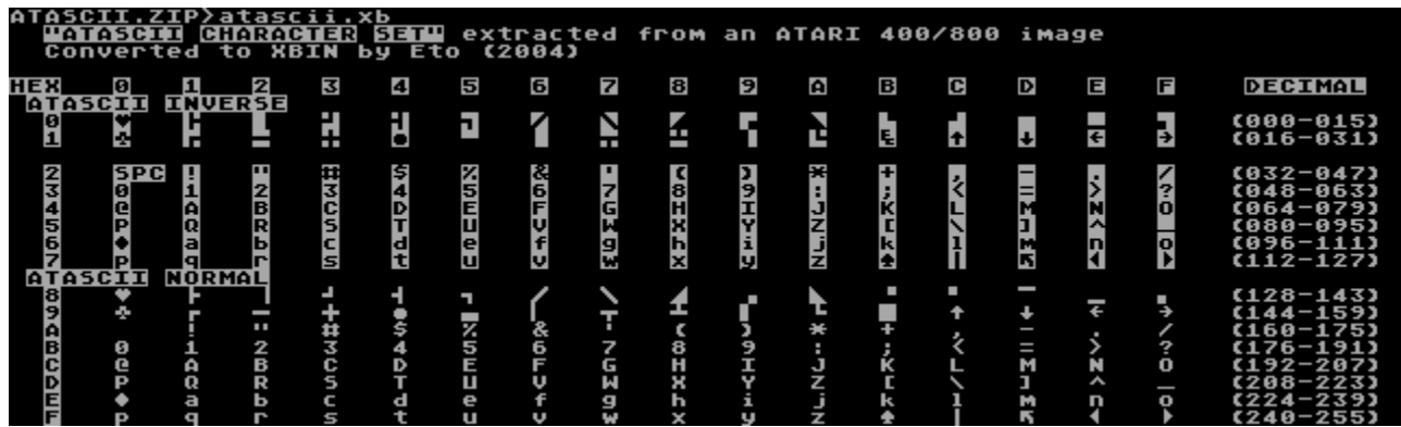
Figure 6. Another character dump of ATASCII glyphs. Note the use of inverse video for headings, as character styling such as bold would be used today.
