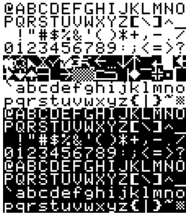
Figure 2. Character dump of the Apple II set, showing normal mode (with MouseText) and inverse video.
