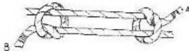
7. FISHERMAN'S KNOT, used to tie two lines or ropes of different sizes together. A knot quickly made and is easy to undo, the ends being simply pulled apart.
