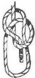
5. THE BOWLINE, a loop that will not slip, to tie round a person being lowered from a building, etc. Form a loop, then in the standing part form a second and smaller loop. Through this pass the end of the large loop and behind the standing part and down through the small loop.
