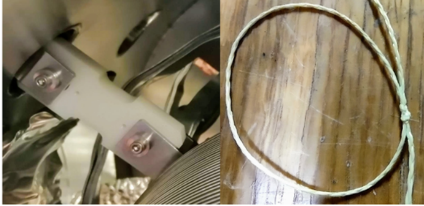
Figure 25 – LHS shows a photograph of the PTFE blocks used in the previous cold bore design compared on the right to the Kevlar string used in the present design.
