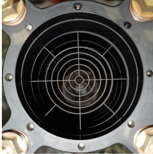
Figure 20 – A photograph of the field ionizer grids. The top two grids are visible in this photograph, the second can be seen by closely examining the upper right hand quadrant.
