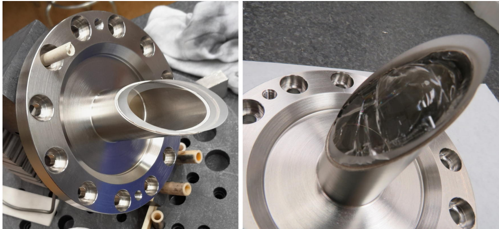
Figure 9 – Photographs of new Brewster window made of UV transparent fused silica vacuum brazed to a titanium flange (left). Result after cryogenic cooldown test (right). The window cracked due to the different thermal expansion coefficients which could not be accommodated despite the thin wall of the inclined tube. Other material combinations are now being studied with the CERN EN-MME-FW group. Photograph by CERN EN-MME-FW group.
