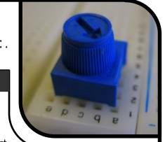
it to a digital number between 0 (0 volts) and 1023 (5 volts) (10 bits of resolution). A very useful device that exploits these inputs is a potentiometer (also called a variable resistor). When it is connected with 5 volts across its outer pins the middle pin will read some value between 0 and 5 volts dependent on the angle to which it is turned (ie. 2.5 volts in the middle). We can then use the returned values as a variable in our program.
