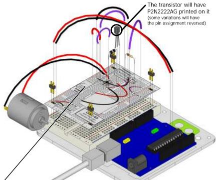
::NOTE: if your arduino is resetting (indicated by a pin13 LED blink), you need to install the optional capacitor:.
