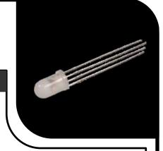
The RGB LED actually has 3 LED elements inside it - Red, Green & Blue. Let's turn these on in combinations to get some brilliant colours out of a single LED!
