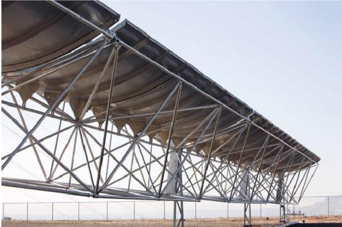
Figure 34: The Skytrough collector (source: Skyfuel)
