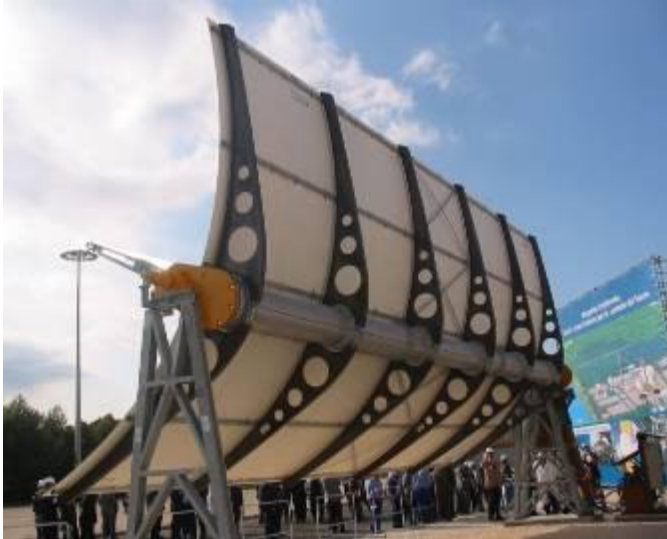
Figure 28: Enea's parabolic trough (source: Geyer, DLR)
