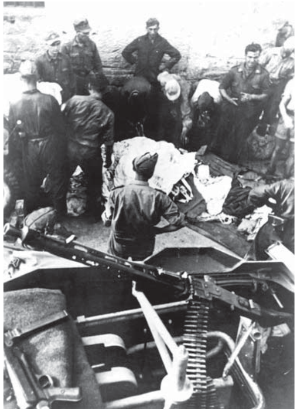
Although the MG 34 was by far the more common weapon for armoured vehicle use, the MG 42 was also used. Here we see an MG 42 mounted on a half-track, by means of a swing-arm mount. (Cody Images)
