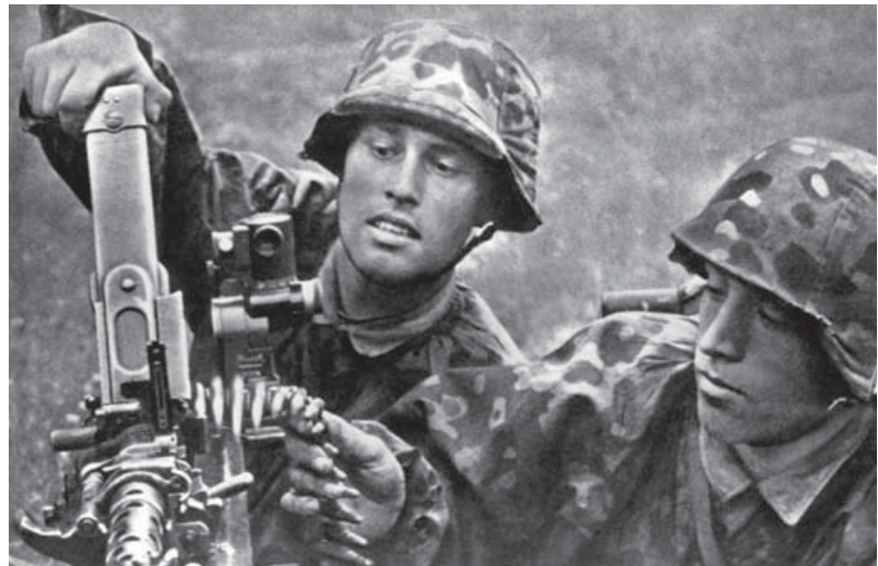
Two Flemish Waffen-SS soldiers load a belt of 7.92mm rounds into an MG 34. Tracers would constitute roughly one in four of the rounds, the others being standard ball or armour-piercing. (Cody Images)
