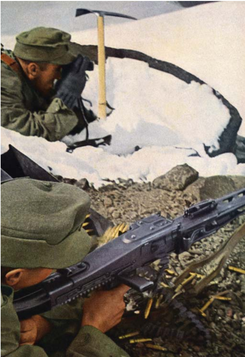
Gebirgsjäger mountain troops fire an MG 42. This weapon has the older style of slab-sided cocking handle, replaced by a vertical bar that gave better cocking grip. (Cody Images)
