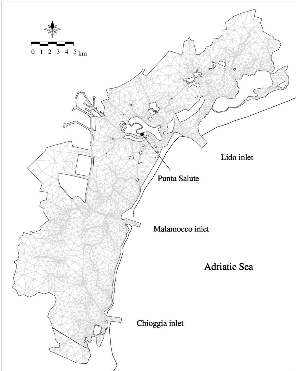
Fig. 1. Overview map of the Venice Lagoon. Indicated are the three inlets and the tide gauge Punta Salute in the city center. Superimposed is the finite element grid used for the simulations.
