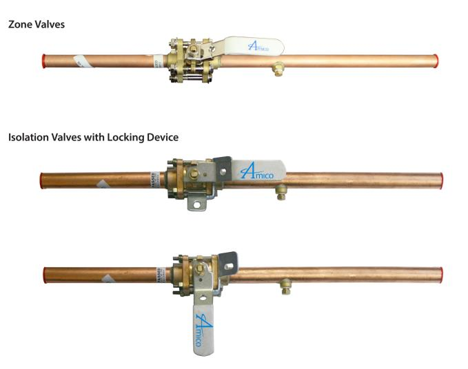
The Zone Valve Shut-offs shall be 3 peice, ball-type design with a brass forging body and a chrome plated, brass ball for sizes 1/2" to 2". Ball seats, stem seals and stem washer shall be reinforced Teflon (PTFE), with Viton stem and flange O-rings. A blow-out proof stem shall be used and the zone shut-off shall have a maximun rating of 600psi (4,137 kPa). All zone shut-offs shall be compatible with pressure medical gases or vacuum service to 29" Hg (98.205 kPa).
