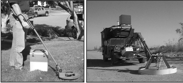
Figure J.1—Present Configuration of the Man-Portable (left) and Vehicle-Mounted NQR Systems (right)
