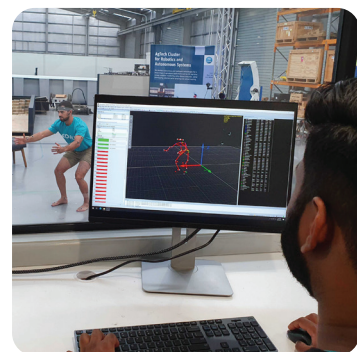
Recording of a patient for range-of-motion analysis using a Webcam and a 3D motion capture system to validate algorithm accuracy. Image courtesy of Coviu.
