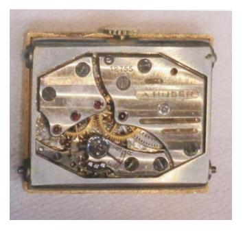
Mechanical movement, the manually-wound LeCoultre caliber no. 410-11U and numbered 12755, produced by LeCoultre in December 1932. It should be noted that the LeCoultre company name has been replaced by "A. HUBER" and that the indication of the number of jewels and the adjustments have also been erased.
