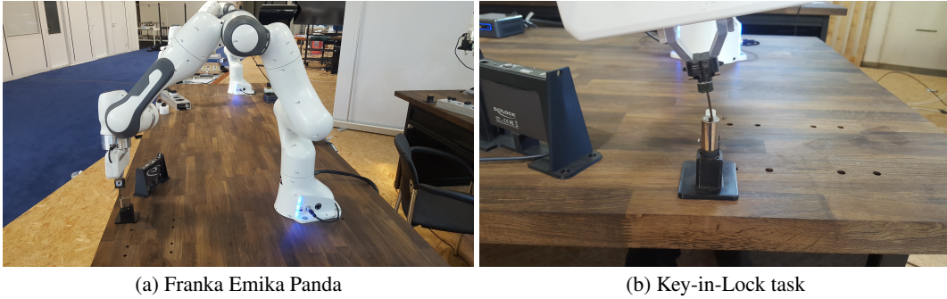
Figure 5: Key-in-Lock experimental setup for validating the multi-level structure learning against state of the art algorithms
