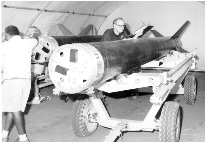
A Black Brant V suborbital rocket motor is prepared for flight during the 1992 El Coqui Campaign. The majority of launches during Coqui Dos will use the single-stage Black Brant V.
