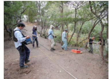
Survey using ground-penetrating radar (GPR) at the Itsukahara Kofun (burial tumulus) site (in Muko City, Kyoto Prefecture)
