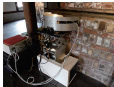
Investigation on brick cultural heritage using portable X-ray diffraction analyzer
