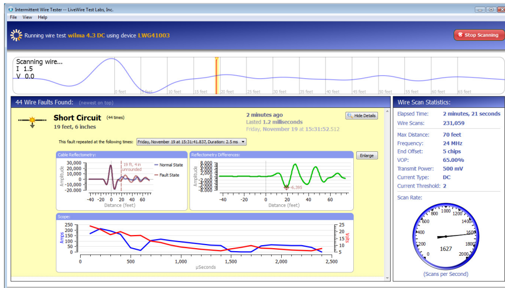
Figure 4: Longer duration 28 VDC arc fault test and graphical result display.
