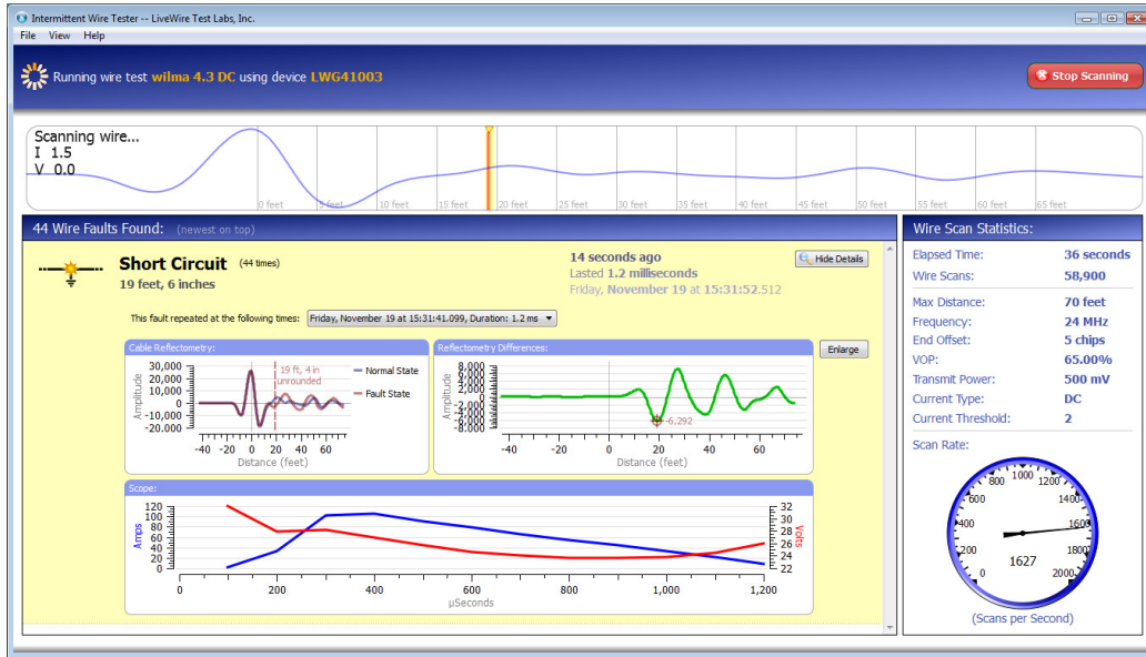
Figure 3: Short duration (1.2 ms) 28 VDC arc fault test and GUI result display.
