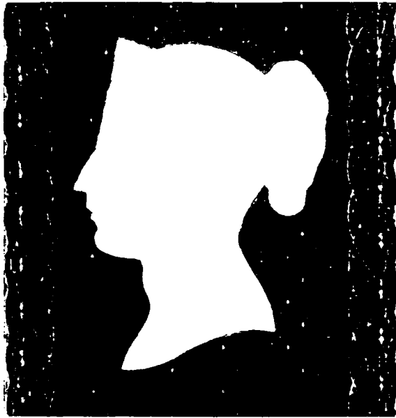
Enlargement showing the effect of the white line on a black ground produced by the Rose-engine upon the roller instead of the flat die.
