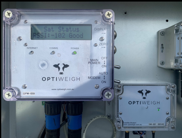
Optiweigh's cattle weighing system sending data via the Swarm satellite network.
