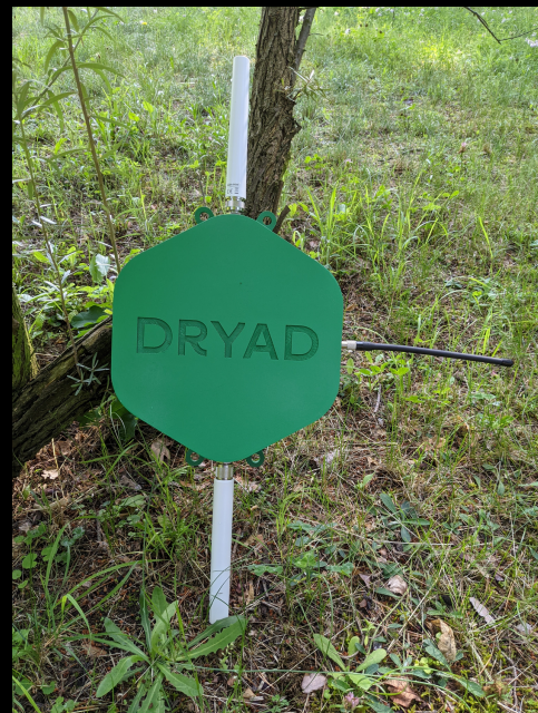
A Dryad gateway with embedded Swarm modem (black Swarm antenna visible)
