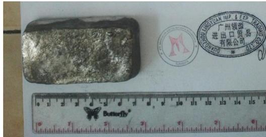
**Gambar 3.2.** Magnesium Ingot
