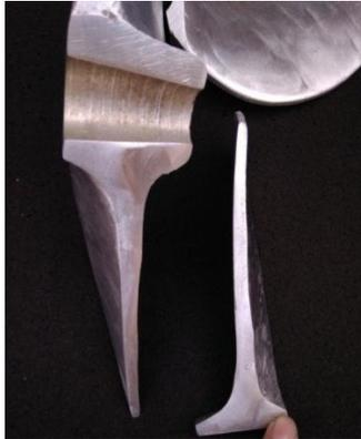
**Gambar 4.7.** Foto Makro *Propeller* paduan Al-Mg potongan melintang
