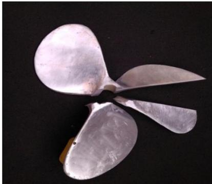
**Gambar 4.5.** Foto Makro *Propeller* paduan Al-Mg tampak depan
