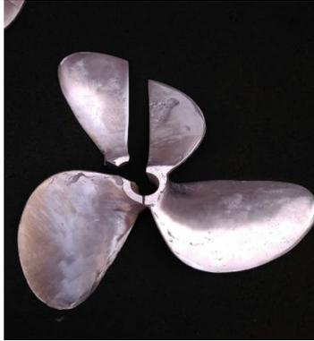
**Gambar 4.2.** Foto Makro *Propeller* paduan Al-Cu tampak depan
