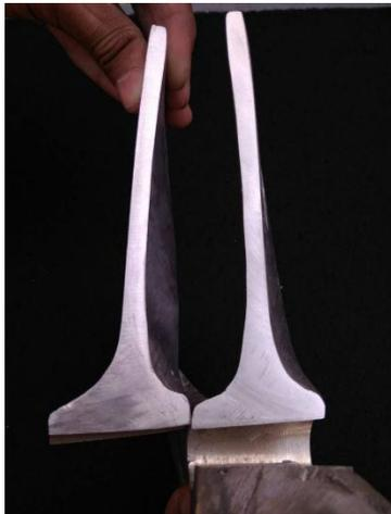
**Gambar 4.3.** Foto Makro *Propeller* paduan Al-Cu potongan melintang
