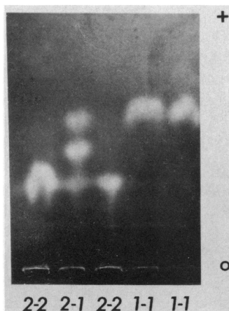
FIG. 2.—Electrophoresis of platelet thrombin-activated, calcium-dependent transglutaminase (factor XIII) (buffer II, 5 hr at 18 v/cm).
