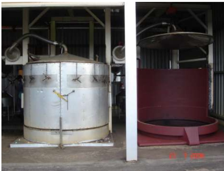
Figure 9.30. A cartridge distillation system at the Former 'Maincamp' property in Australia. (Photo courtesy Mr. John Bax).
