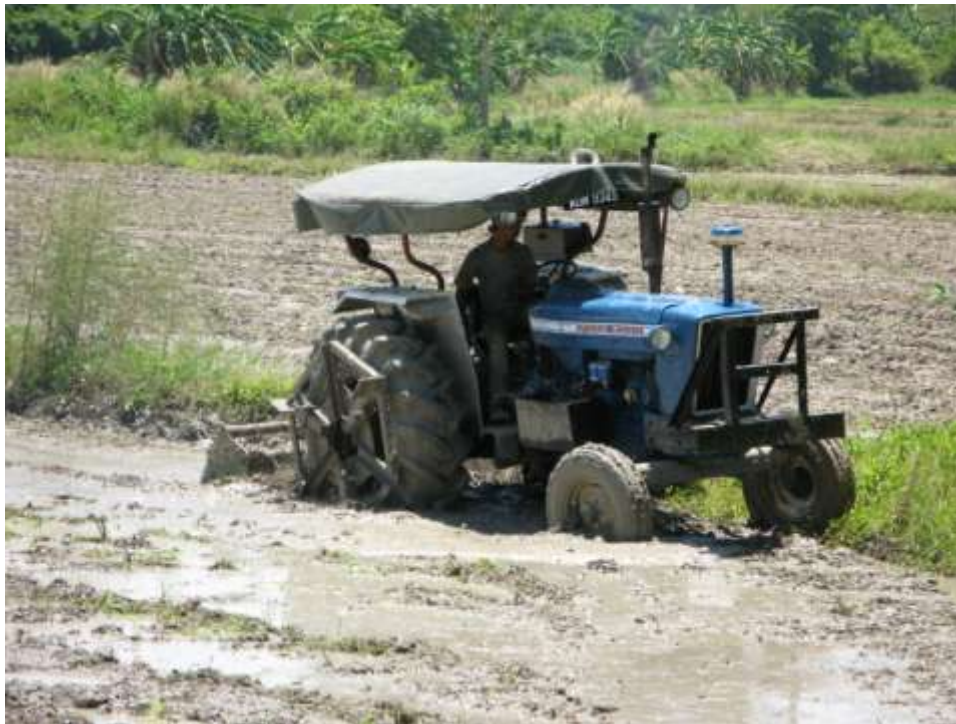
Figure 9.22. Paddle arrangement connected to tractor wheel for 'boggy' conditions.
