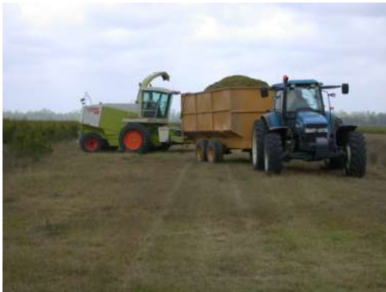
Figure 3.1. The tea tree harvester and bio-mass collection bin towed by a tractor at the former “Maincamp” plantation (Photo courtesy of Mr. John Bax) [6]
