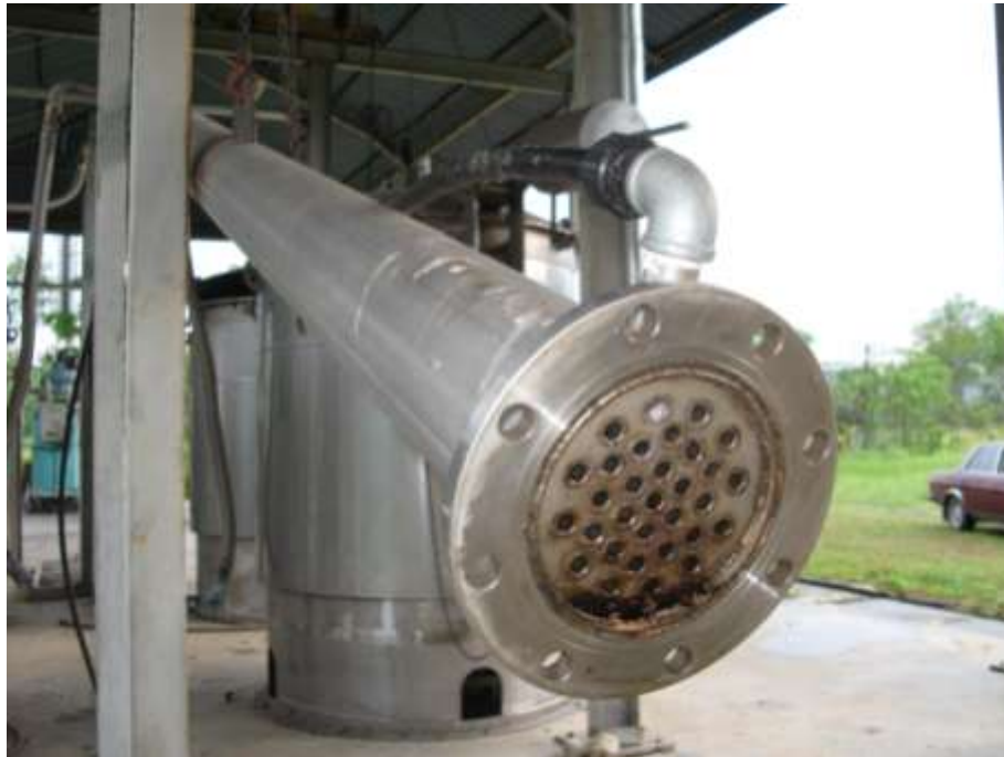
Figure 5.10. Photo showing the condenser with the end manifold removed to expose the internal cooling pipes at the Author's property in Perlis, Malaysia.
