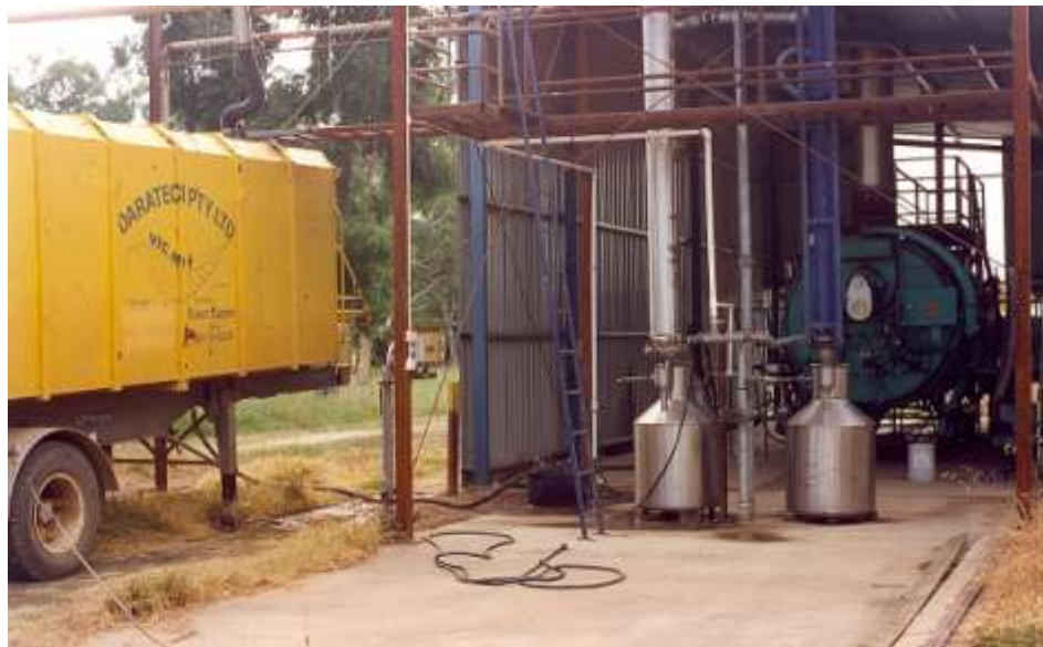
Figure 9.31. Box coupled to the steam source at the distillery for peppermint Distillation at Myrtleford, Victoria (Photo courtesy of Mr. Fred Bienvenu).
