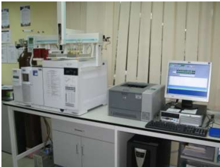
Figure 4.12. A Gas Chromatograph-Mass Spectrometer (GC-MS) The Forest Research Institute of Malaysia (FRIM) in Kuala Lumpur, Malaysia.
