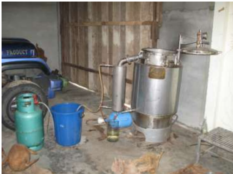
Figure 3.5. A small distillery in Trang for the extraction of oil from wild collected Cinnamomum species.
