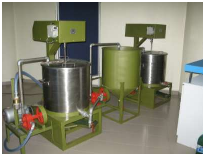
Figure 9.25. A small plant designed and built by The Author to convert used cooking oil to bio-diesel.
