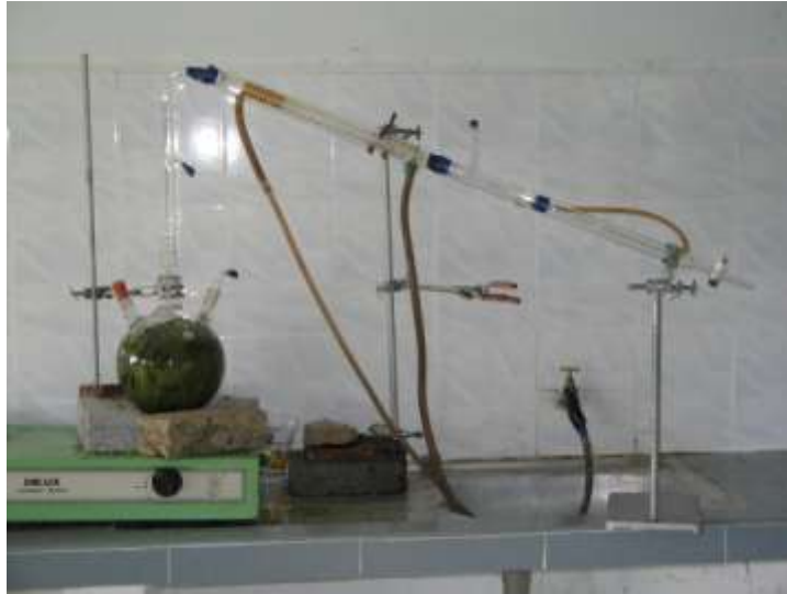
Figure 9.26. A glassware still is usually more efficient than a commercial still.
