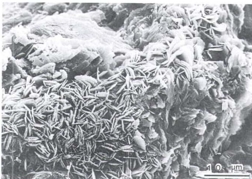
Authigenic chlorite forms a partial coating on a detrital framework grain. Surface sample of Point Lookout sandstone, La Plata Co., CO. Photo donated by Bill Keighin.
