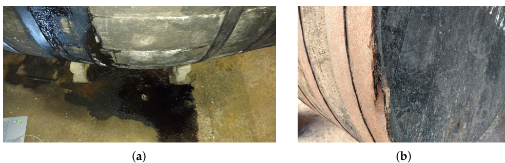
Figure 12. Defective casks. (a) Cask losing wine through small cracks. (b) Defective cask due to a received blow.
