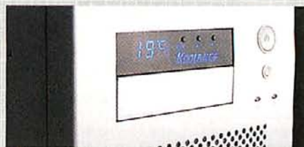
▲ A quick glance at the front-mounting panel tells how cool it is under the hood.
