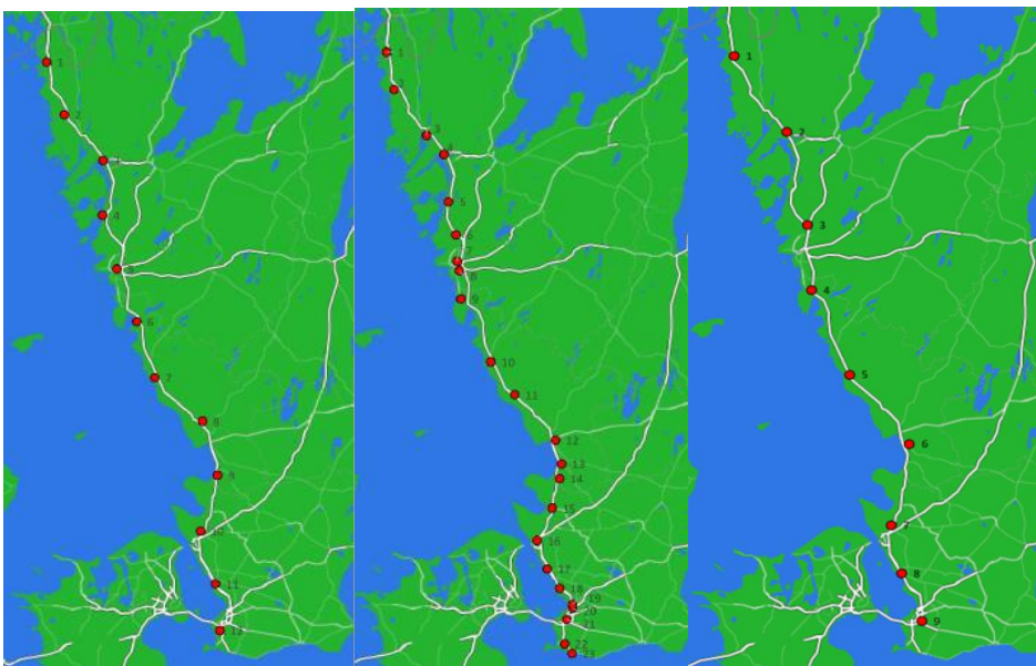
Figure 11: The placement of substations along E6 assuming a substation every 40 km (left), optimization according to load (center) and using existing grid to as large extent as possible (right). All cases assume 100 % electrification of the heavy vehicles using E6.
