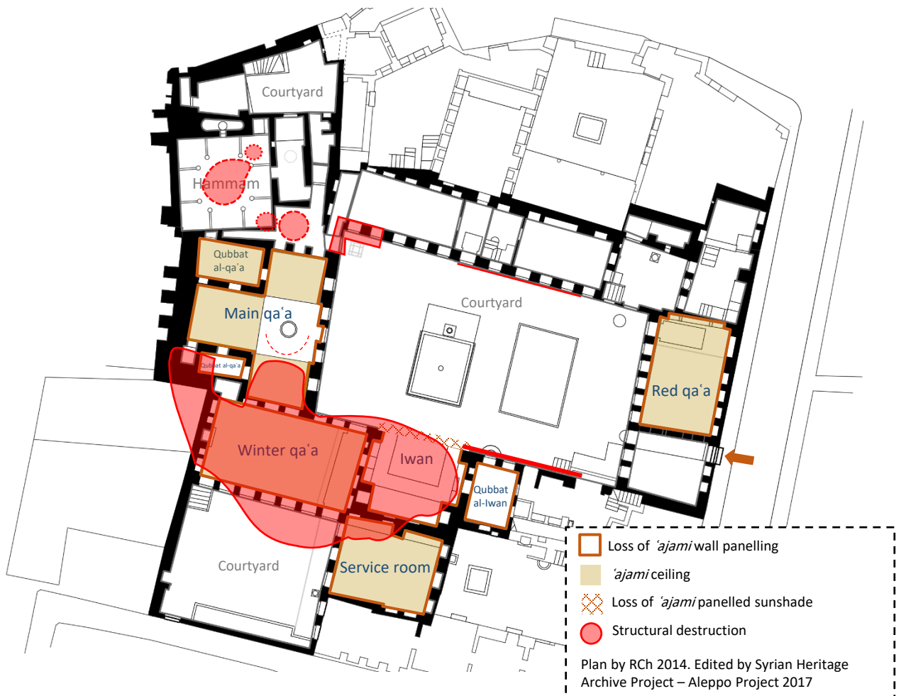
Figure 13: The location of removed 'ajami panellings with structural destruction
