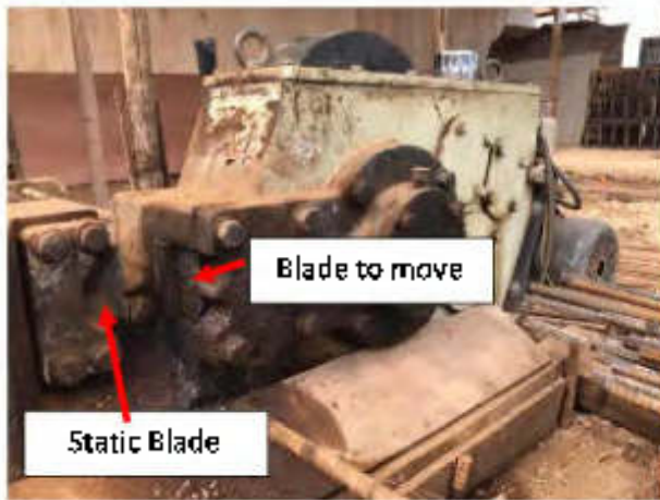
Rebar Position and Pinch Point
