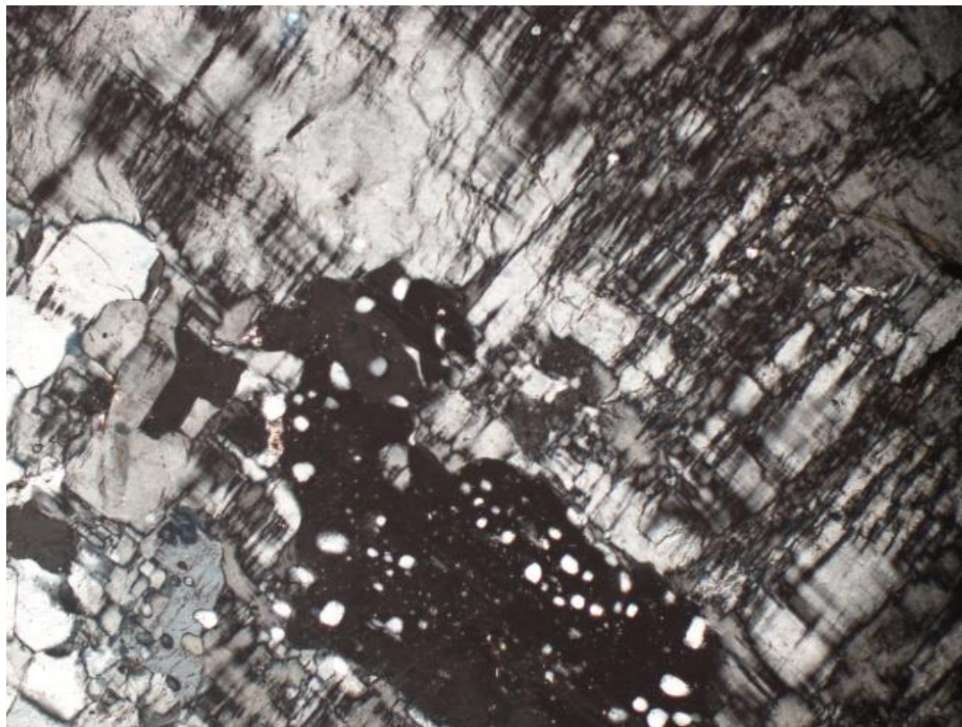
Figure 5. Photomicrograph of Marinette Quartz Diorite, showing myrmekite (black with white quartz blebs) adjacent to microcline (cross-hatched twinning, dark gray and white). Quartz grains outside microcline (white and cream).
