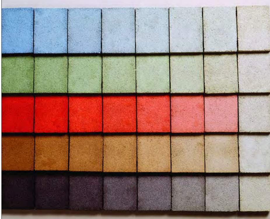
These concrete samples show the impact of pigment dosage rates. The chips on the right are plain, uncolored concrete while the chips at the left are approaching the color saturation points of the pigments. Even low dosage rates can make a profound difference on the appearance of concrete and are an economical way to add value to decorative concrete.
