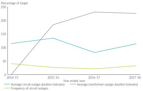
This view shows, in general, the PWC Network is performing within acceptable limits since the average circuit outage duration (ACOD) and frequency of circuit outages (FCO) are safely below the target. The current targets were approved by the commission in July 2013 for the current determination period from 1 July 2014 to 30 June 2019.
