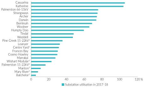
Figure 18: Substation utilisation in N-1 conditions on 2017-18 Darwin-Katherine (POE 10)
