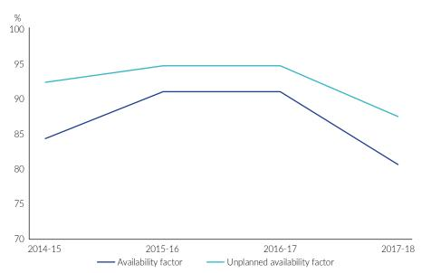
Figure 27: Capacity weighted average availability factor for Alice Springs generating units
