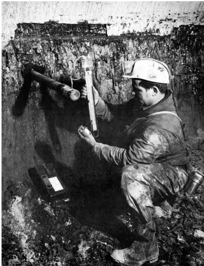
Measuring the outflow of methane gas from a horizontal hole drilled into an unmined coal seam. (photo credit: Bureau of Mines publication)
