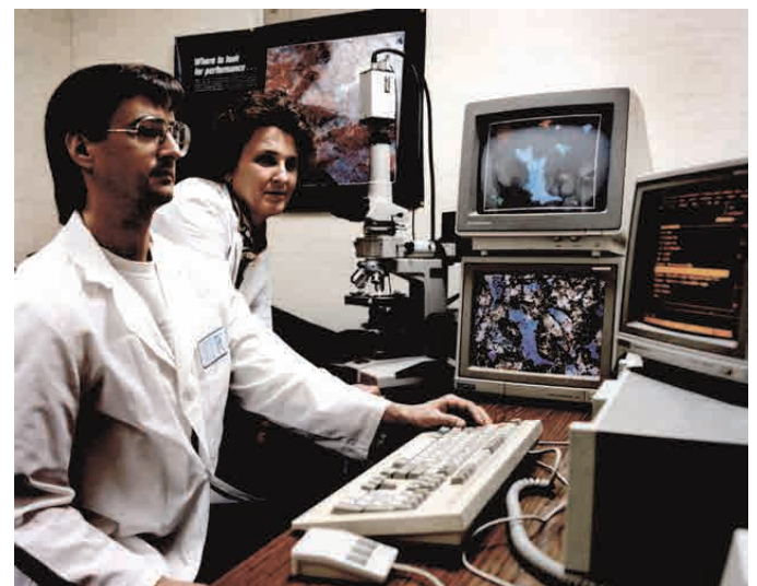
Susan Jackson and Alan Brinkmeyer examine magnified images of petroleum reservoir rock samples using a petrographic analyzer.
