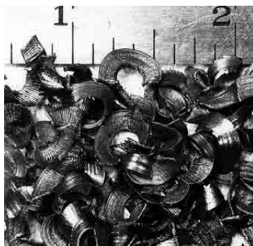
Steel lathe turnings proved to be effective as catalyst material for experimental Fischer-Tropsch reactors. (photo credit: National Archives and Records Administration)
