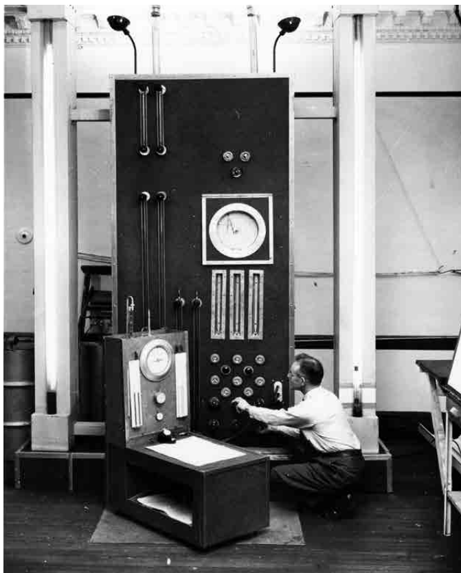
E. M. Tignor adjusting the controls of a model oil well in the field office at Franklin, Pennsylvania.
