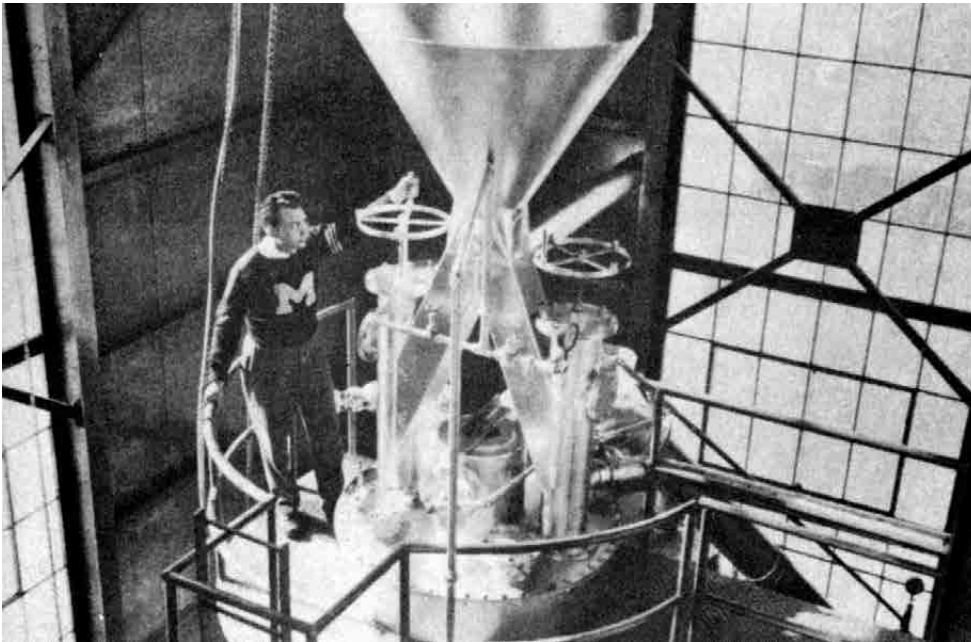
Interior view of the retort building at the Grand Forks gasification plant, showing the hopper and charging valves that fed lignite into the top of the Reyerson-Gernes water-gas generator. (photo credit: Bureau of Mines publication)
