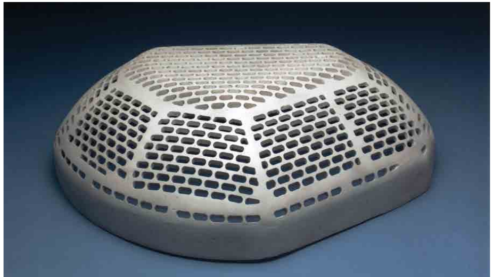
The cast steel armor program at Albany produced this three-piece bustle to protect the rear of the turret and the commander's hatch on the Army's Bradley Fighting Vehicle. The angled slots in the armor are designed to fracture incoming projectiles into numerous pieces, none of which has enough energy to penetrate the vehicle.
