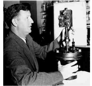
Wilburn C. Schroeder displaying the embrittlement detector that the Bureau of Mines invented to help protect against boiler failures. The Bureau received a patent for this device in July 1943. (photo credit: National Archives and Records Administration)
