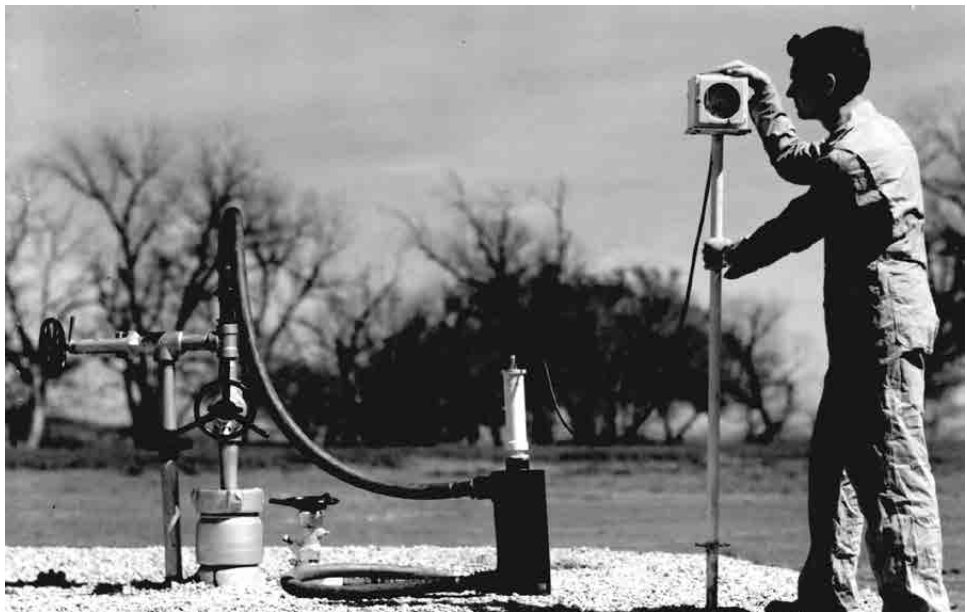
A Bartlesville engineer using field instrumentation to detect the flow of low-level radioactive tracers underground.
