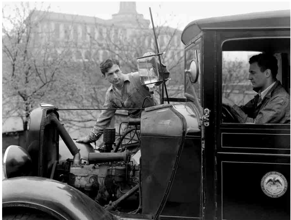
A Bureau of Mines truck equipped to run on synthetic gasoline derived from coal, 1941. (photo credit: National Archives and Records Administration)
