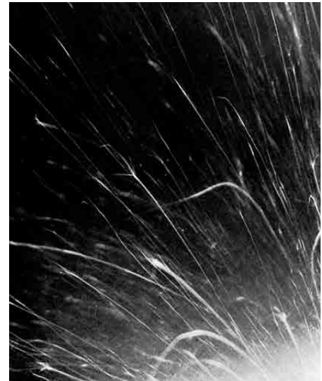
High-speed photography revealed branching patterns in the paths of sparks thrown off by an explosion. (photo credit: Bureau of Mines publication)
