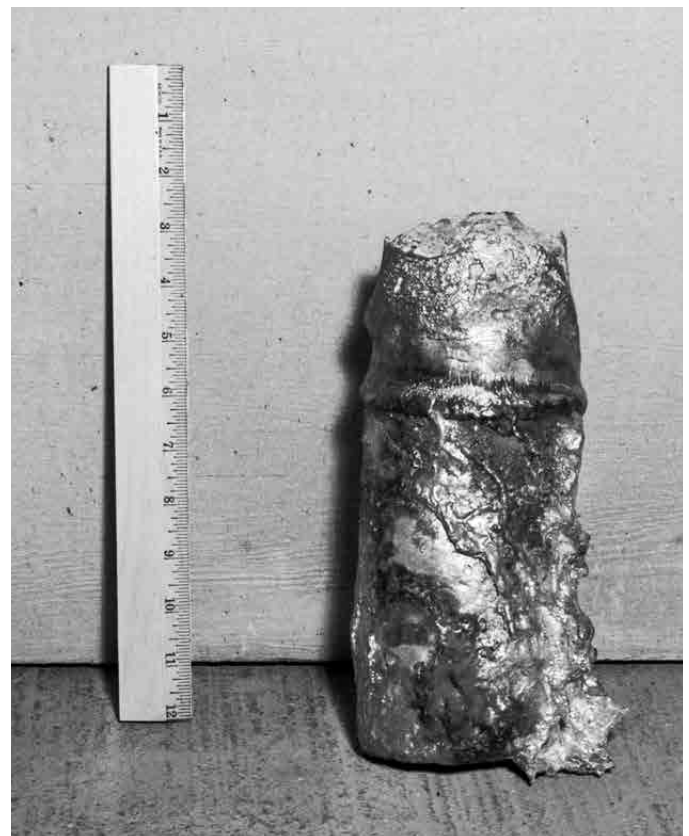
Mass of molybdenum metal made using the metal bomb reduction process
