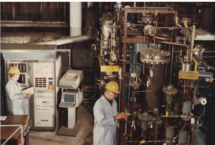
An experimental hot-gas cleanup system at METC in the mid-1980s. Using zinc ferrite as a sorbent, this system could remove up to 99.9 percent of the sulfur from a stream of hot synthesis gas or fuel gas.
