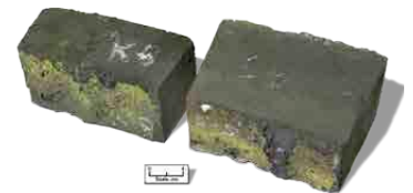
Comparison of chromia refractory bricks, with NETL's formulation (right) showing much less wear than the standard commercial brick (left).
