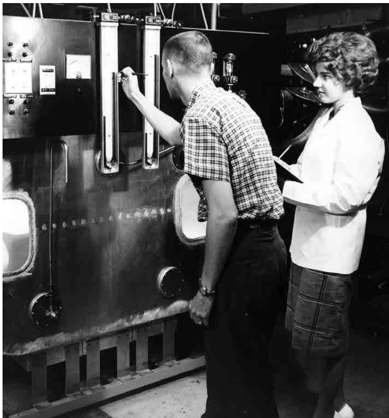
Don Merckling and Patricia Simpson take a pressure reading on Hurn's smog chamber, 1961.
