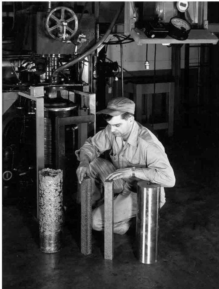
Albany employee showing the various stages of zirconium from sponge (left) to pressed sponges (middle) to an ingot (right).
