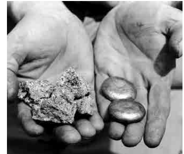
Yttrium sponge (left) and ductile yttrium buttons first made at Albany in 1959.
