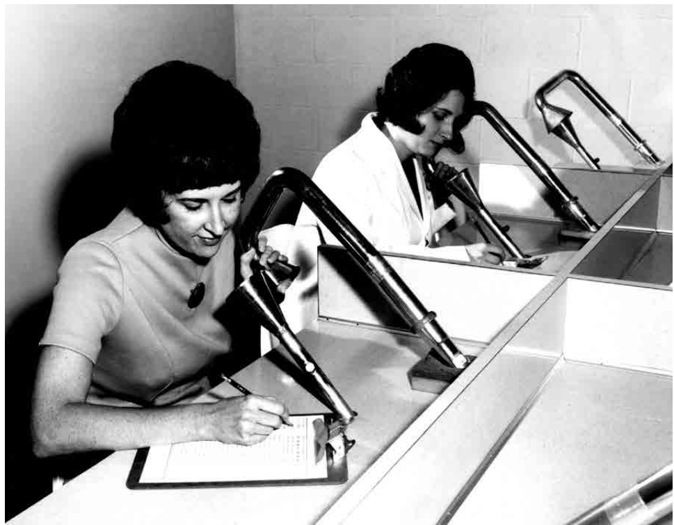
Two Bartlesville women with highly sensitive noses evaluate the characteristics of diluted diesel fumes.
