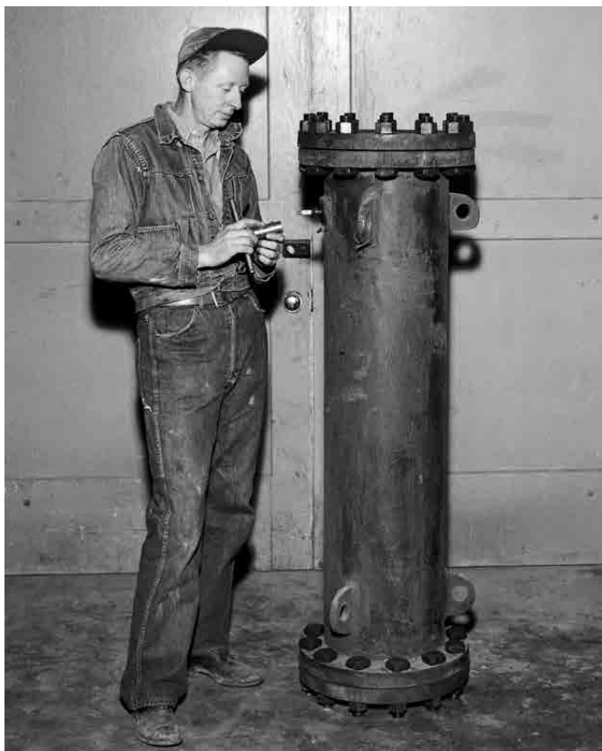
Emil Anderson, a Bureau equipment mechanic, works on a reactor for the metal bomb reduction process.
