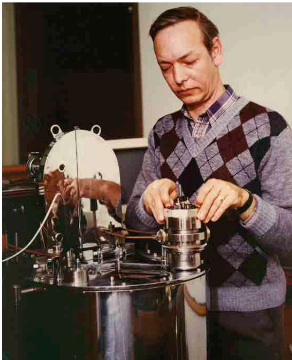
Bill Steele of Bartlesville setting up a thermodynamics experiment using the rotating bomb calorimeter in the 1980s.
