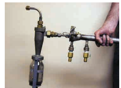
Close-up picture of the “Thief” apparatus used to extract partially-combusted coal from NETL's pilot-scale combustor
