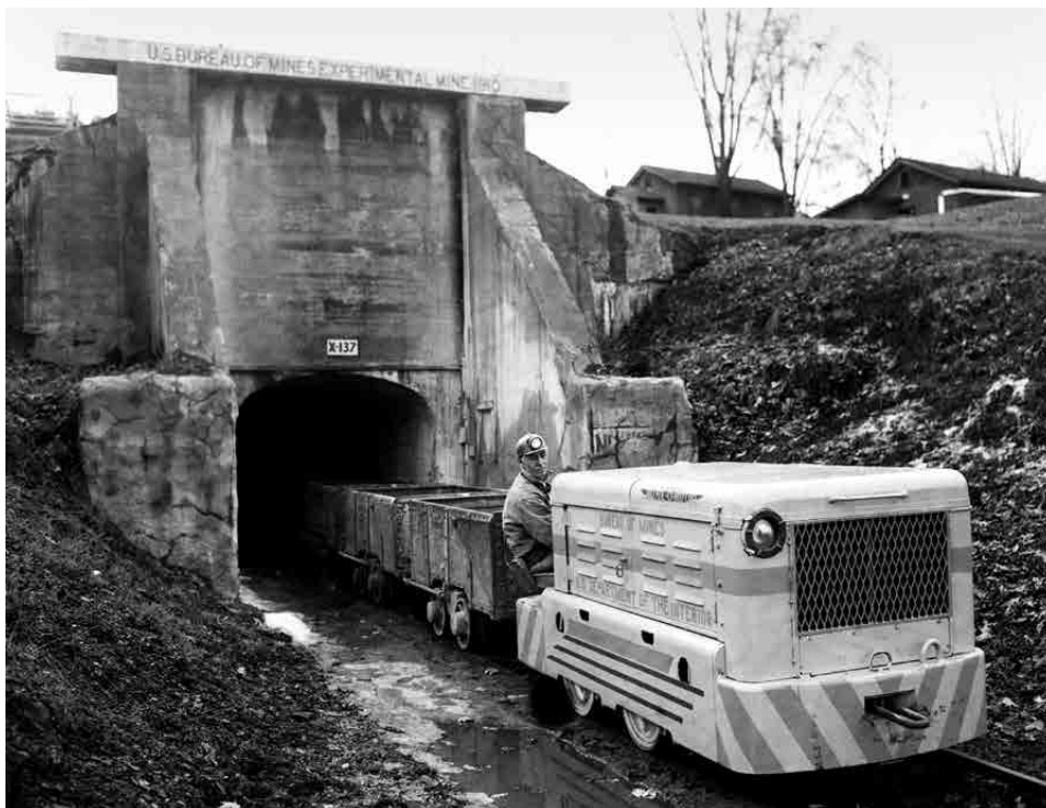
By 1955, permissible diesel engines had replaced mule power on the Experimental Mine's underground tracks. (photo credit: National Archives and Records Administration)
