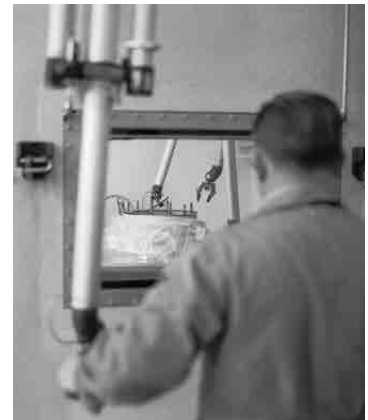
Scientist operates robotic arms to manipulate a rod in Albany's hot cell, 1962.
