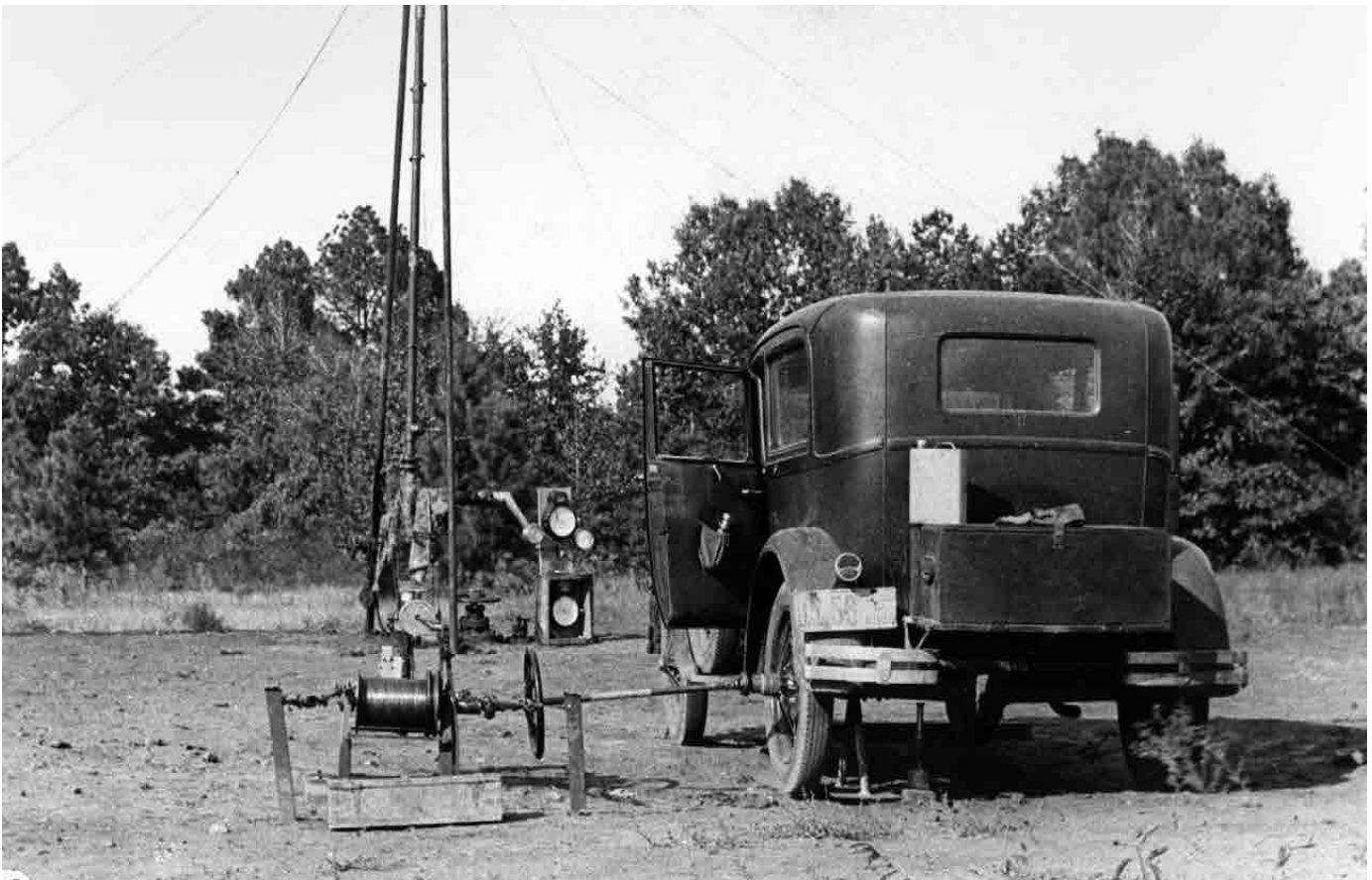
A 1929 Model A Ford coupled to a device to lower a bottom-hole sampler into a well. (Bartlesville, 1932)
