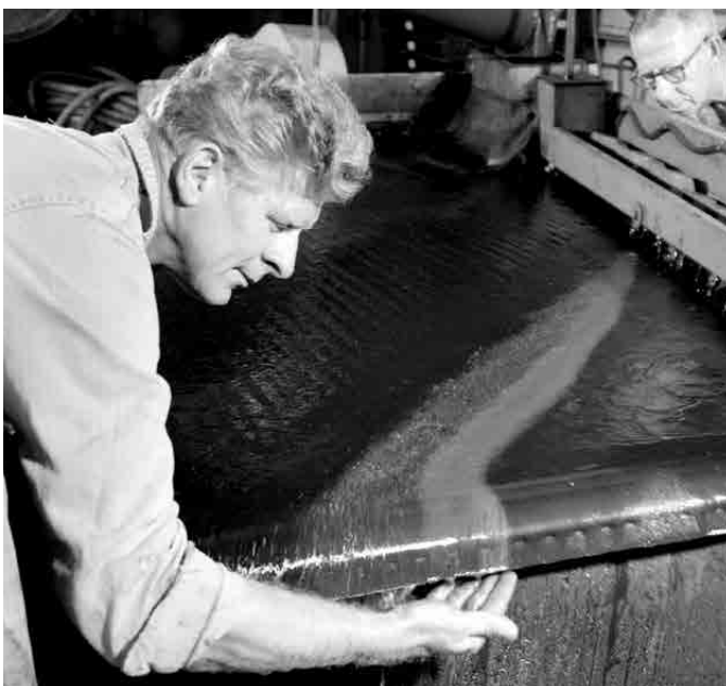
A wet concentrating table for separating sulfur-containing pyrite from coal. (photo credit: National Archives and Records Administration)
