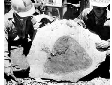
A large block of spent oil shale after an above-ground retorting experiment, 1967. Light areas were oxidized during heating and combustion, while the dark center area still contains unreacted residual carbon. This block originally weighed about 650 pounds. (photo credit: Bureau of Mines publication)
