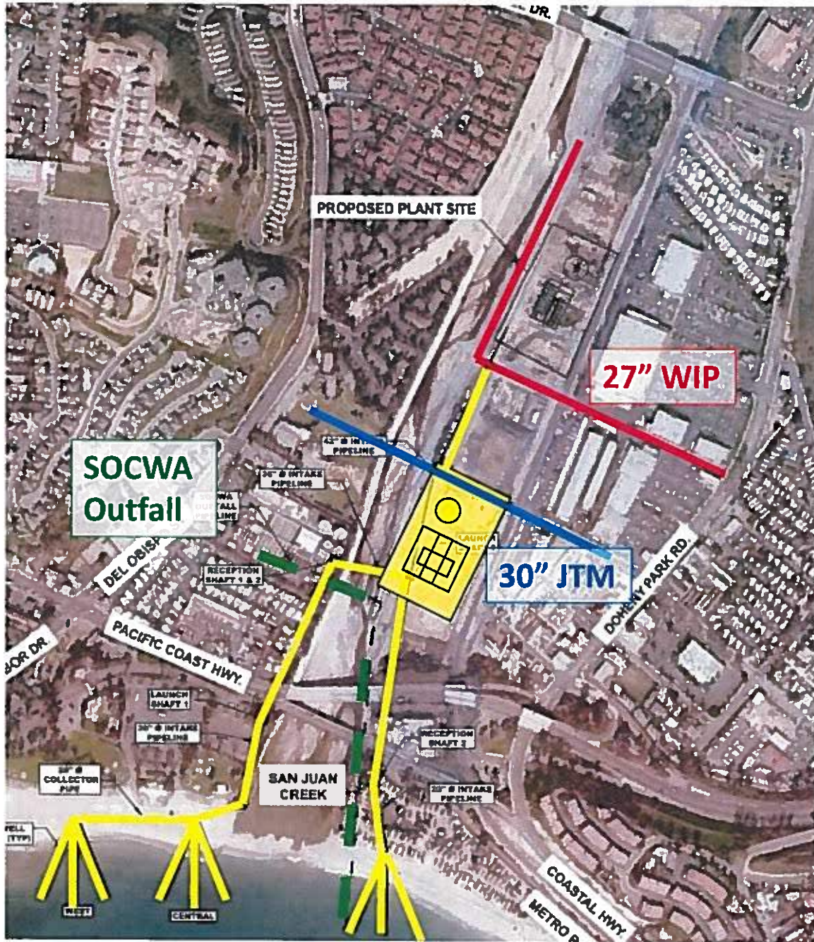
Figure 1B - Schematic of Doheny Desal Project Layout
