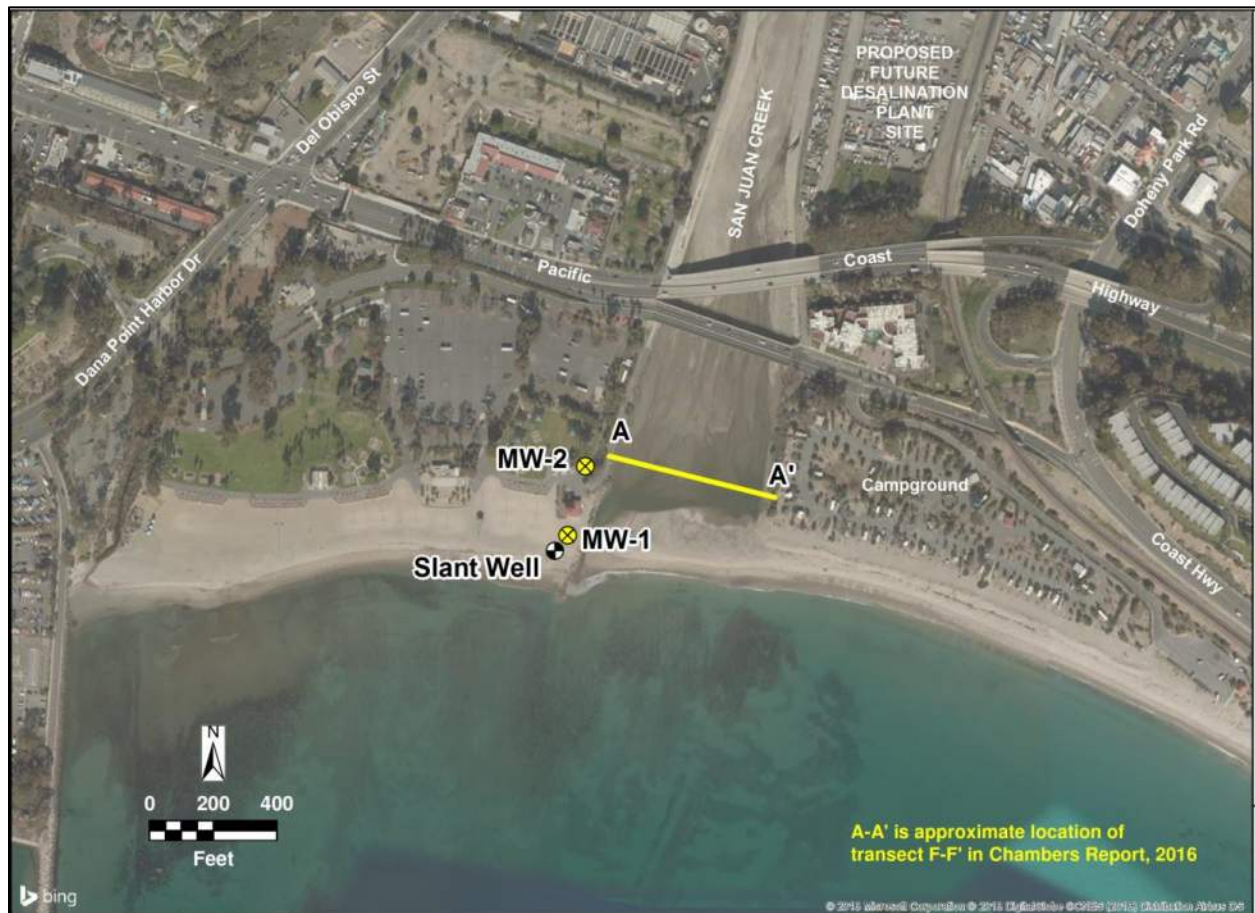
Figure 2-1. Monitoring Well Locations in the Vicinity of the San Juan Creek Lagoon
