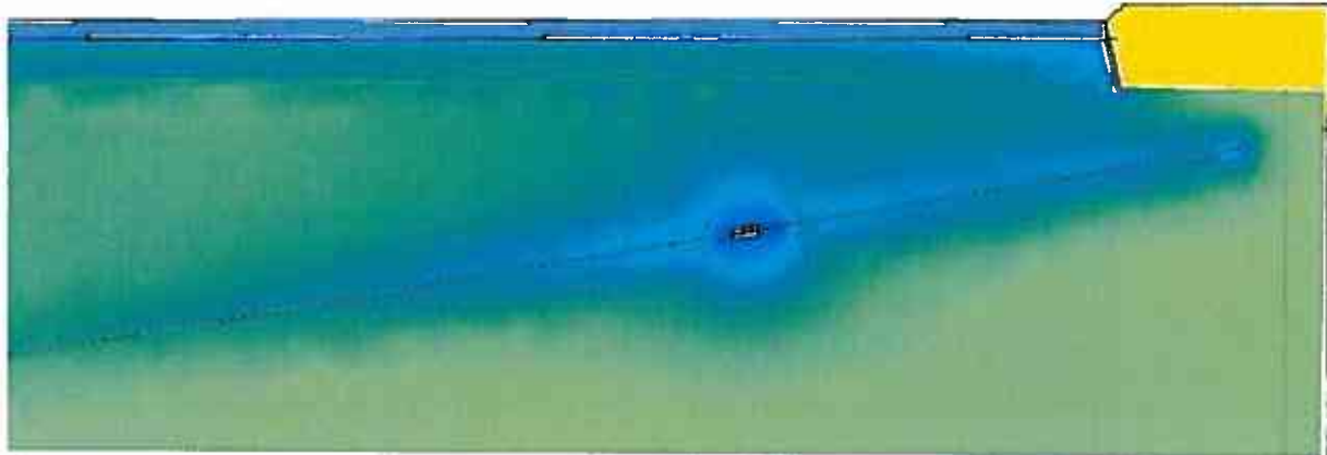
Figure 3. Zoomed-in suction zone above the slant well from Figure 2. The flux of DOM, SOM, POM matter will follow the infiltration path of water and will eventually be adsorbed and immobilized. That organic matter becomes a nutrient for anaerobic bacteria producing hydrogen sulfide. The infiltration zone depends on the submersible pump capacity, however my preliminary modeling shows that one can expect DOM and SOM concentrations at least two orders of magnitude higher than in natural fluxes caused by advective waves actions. As can be seen by the color scale, colloids will deposit in the entire filter strata and there is more DOM and SOM above and in the direct vicinity of the slant well.
