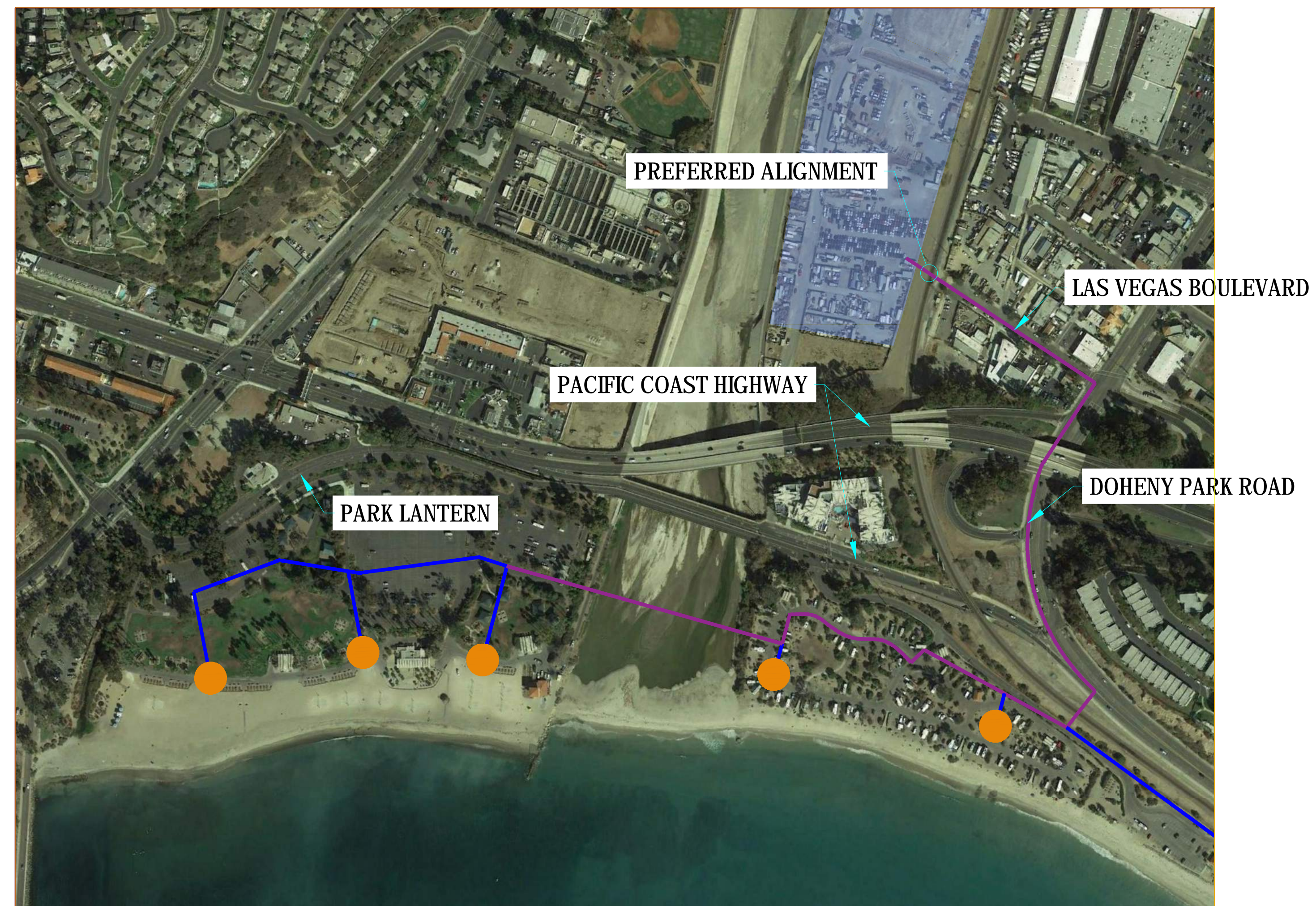
3 RAW WATER CONVEYANCE LAYOUT - PREFERRED ALIGNMENT 1" = 270'
