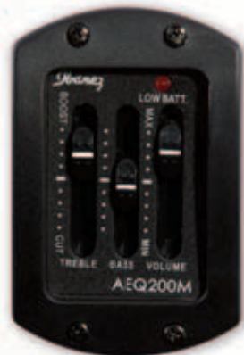
Ibanez AP2 magnetic soundhole pickup and AEQ200M preamp with 2-Band EQ on TCM50VBS.
