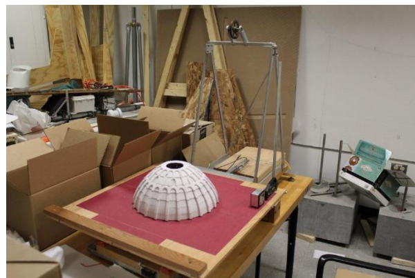
Figure 7: The 3D printed dome on the tilt table. The smallest pieces on the top row have been removed for ease of construction.
