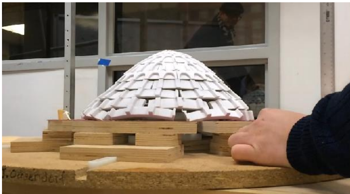
Figure 9: The screen capture from a video of the test reveals the collapse mechanism of the dome. It can clearly be seen that the lower pieces have rotated and some of the upper pieces have slid on top of each other.
