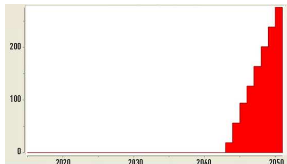
FIG. 13(d). SNF accumulation (in tons) from PWR Generic NGS I (candidate NPP) in dry storage for high scenario.
