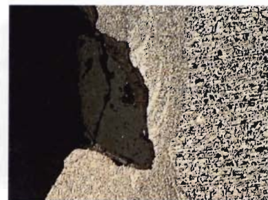
Figure 6.15 Weld root slag inclusion at 8 o'clock position
