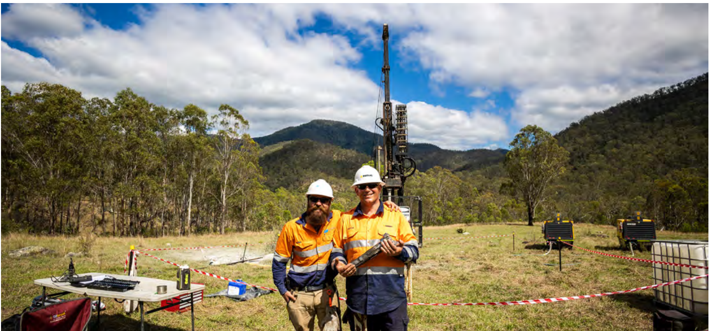
Photo - Geotechnical investigations completed near the project's proposed lower reservoir.
