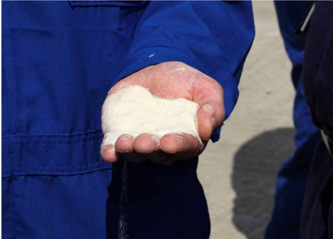
Photo 5.17 - Sand used in hydraulic fracturing operation in Bradford County, PA.
