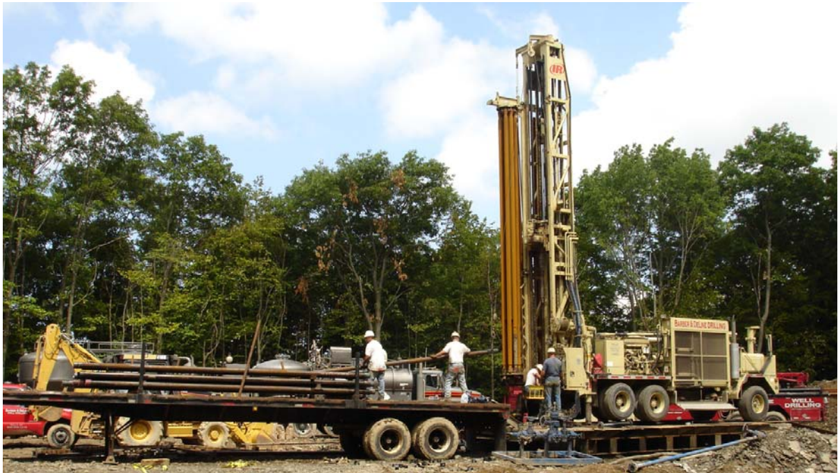
Photo 5.15 Top Drive Single. Barber and DeLine rig, Sheckells 1, Town of Cherry Valley, Otsego County. Credit: NYS DEC 2007.
