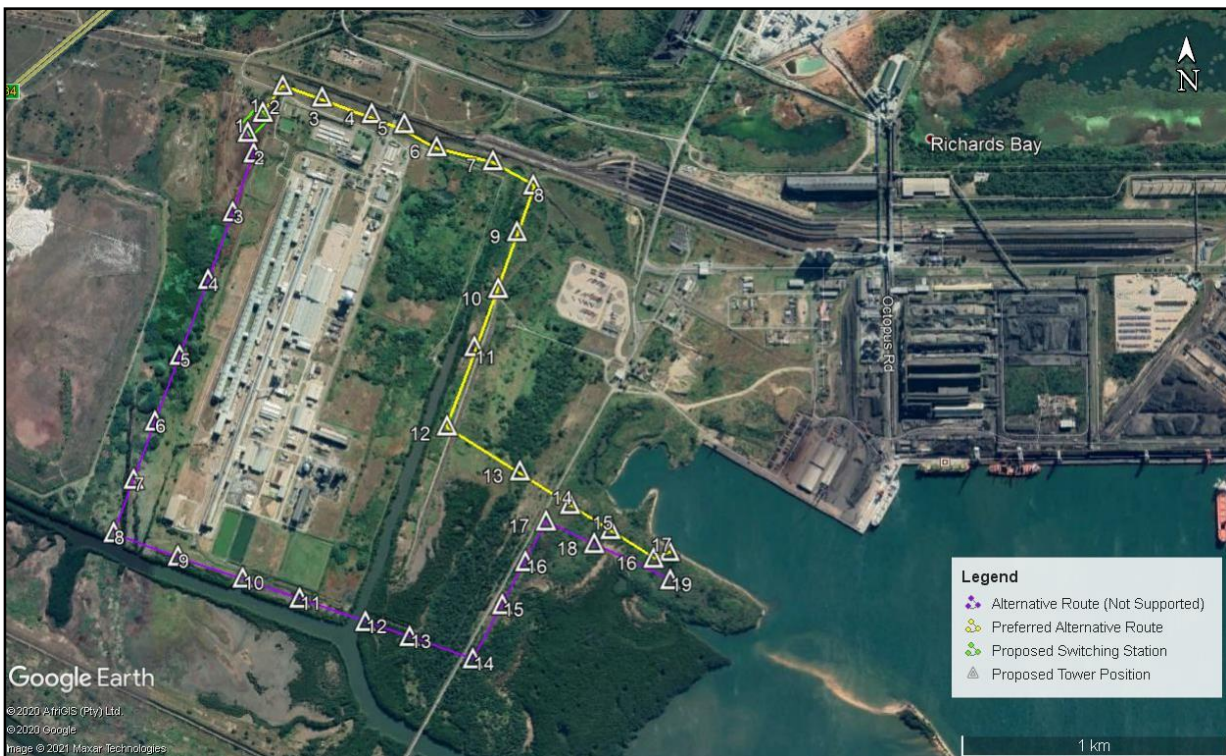
Figure 9-4: Transmission line route alternatives from the Powerships to the proposed switching station – Preferred Alternative (yellow) and Alternative 2 (purple).
