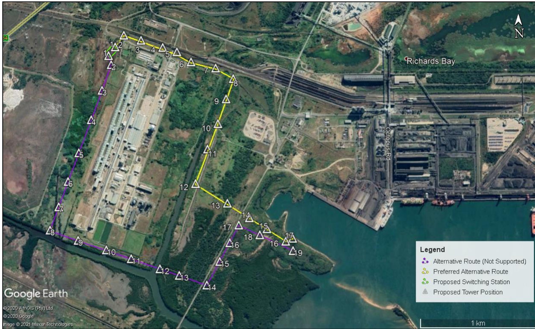
Figure 3-7: Transmission line route alternatives from the Powerships to the proposed switching station – Alternative 1 (yellow) and Alternative 2 (purple).
