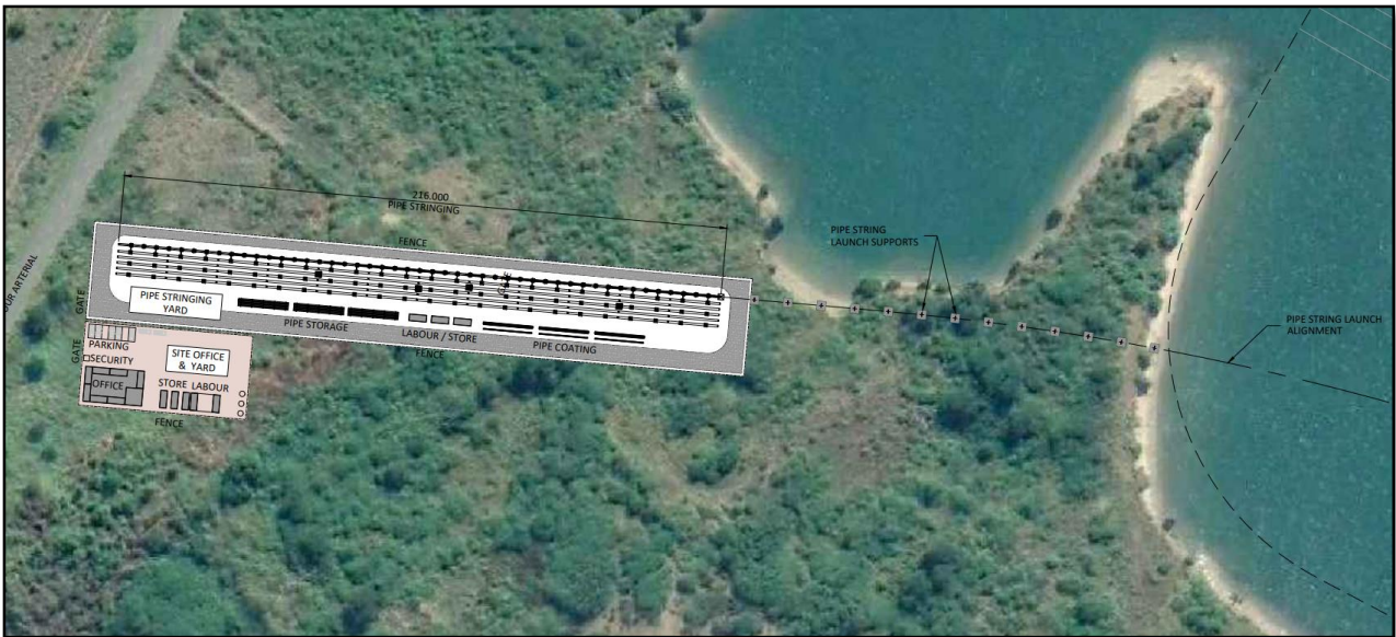
Figure 3-5: Proposed location for the temporary laydown area for the installation of the gas pipeline.
